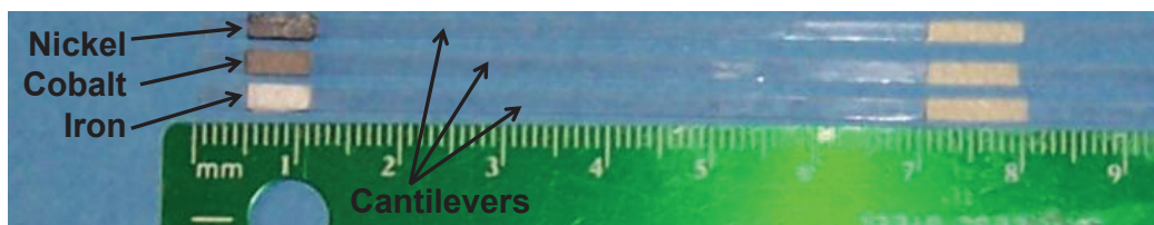
Figure 4.11. Image shows plastic cantilevers coated with 1mm thick ferromagnetic nickel, cobalt and iron gels.
