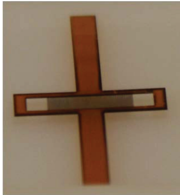
Figure 5.8. Laser machined IDC structure on Kapton film.
