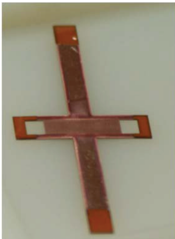
Figure 5.9. Copper deposited IDC on Kapton film.
