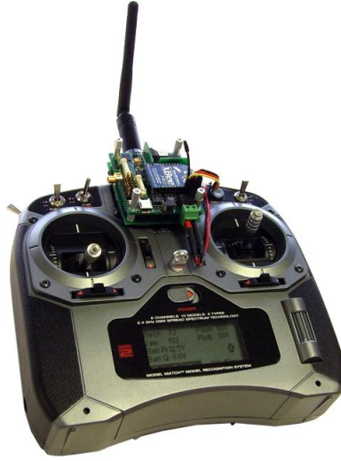
Figure 31. A second quadrotor sensor board detects the pilot's orientation
