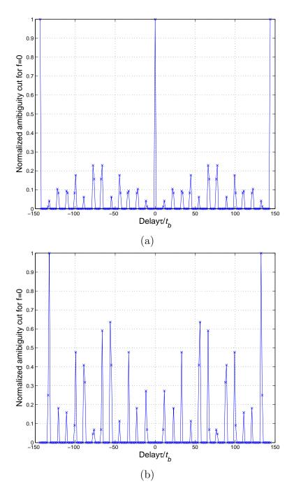
Figure 3.7. (a)Periodic autocorrelation property of 144-length optimized punctured ZCZ sequence-pair  $(x_1, y_1)$  (b)Periodic cross correlation property of 144-length optimized punctured ZCZ sequence-pair  $(x_1, y_2)$ .
