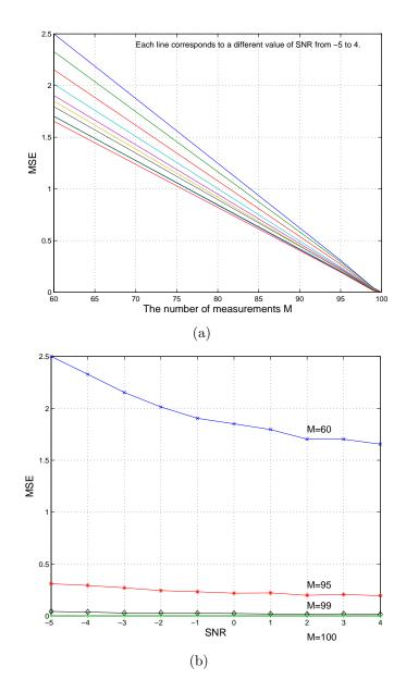
Figure 10.4. Normalized MSE between reconstructed signal and original signal for fixed N = 100: (a) Normalized MSE versus M; (b) Normalized MSE versus SNR.
