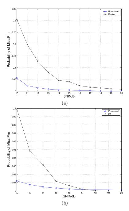
Figure 4.6. Probability of miss targets detection for 31-length Punctured binary sequence-pair VS. 31-length P4 code: (a) No time delay, Doppler shift is less than 1; (b) Time delay, Doppler shift is less than 1..
