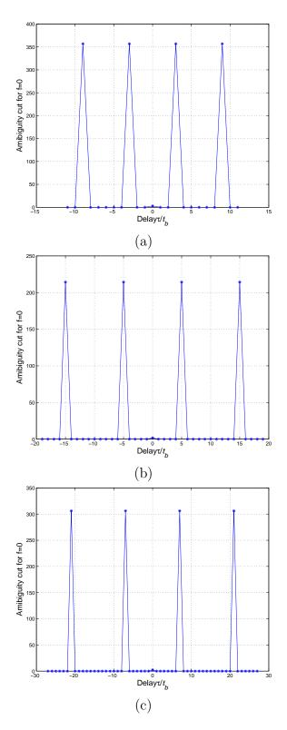
Figure 7.4. Range Resolution:(a) 12x4 ZCZ codes;(b) 20x4 ZCZ codes;(c) 28x4 ZCZ codes.
