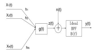
Figure 8.1. Radar sensor network channel model.
