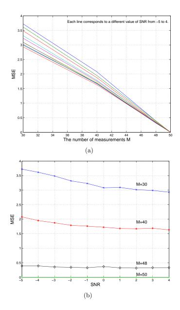
Figure 10.5. Normalized MSE between reconstructed signal and original signal for fixed N = 50: (a) Normalized MSE versus M; (b) Normalized MSE versus SNR.
