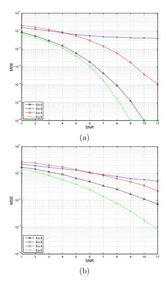
Figure 7.5. MSE of beamforming at the receiver within the first model: (a) Nonfluctuating model; (b) Fluctuating model .
