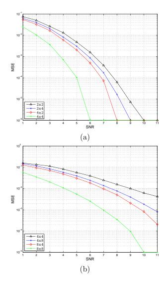
Figure 7.6. MSE of beamforming at the receiver within the second model: (a) Non-fluctuating model; (b) Fluctuating model .
