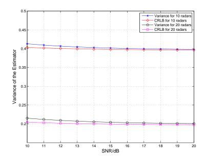
Figure 10.6. Variance of RCS ML estimator with different number of radars in RSN (The actual RCS parameter  $\theta = 2$ ).
