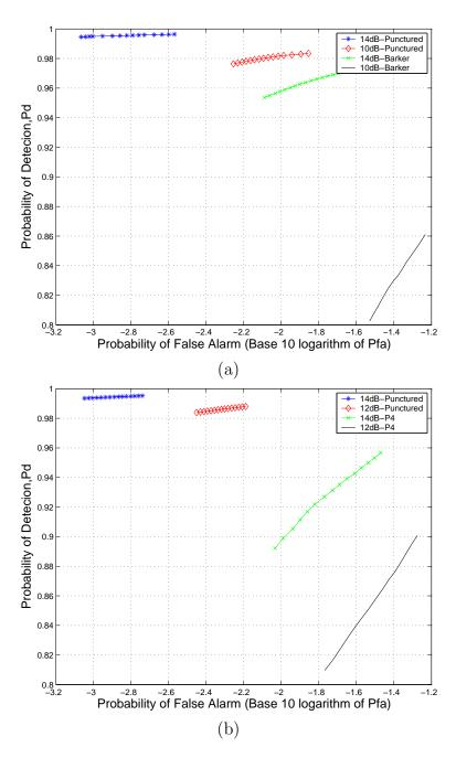
Figure 4.7. Probability of detection versus probability of false alarm of the coherent receiver for 31-length Punctured binary sequence-pair VS. 31-length P4 code: (a) No time delay, Doppler shift is less than 1; (b) Time delay, Doppler shift is less than 1.
