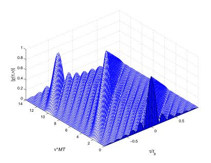
Figure 10.2. Ambiguity function of Stepped-Frequency train of unmodulated pulses.
