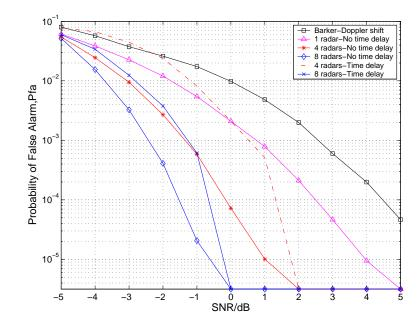
Figure 5.3. Probability of false alarm in RSN under the condition of no time delay but Doppler shift or time delay and Doppler shift .
