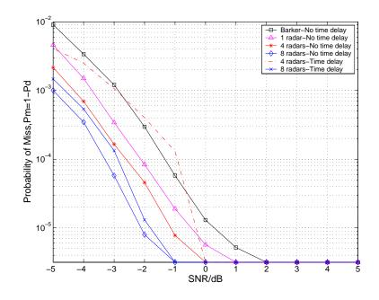
Figure 5.2. Probability of miss detection in RSN under the condition of no time delay but Doppler shift or time delay and Doppler shift.
