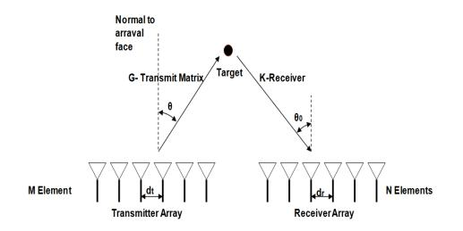
Figure 7.1. MIMO Radar Model.
