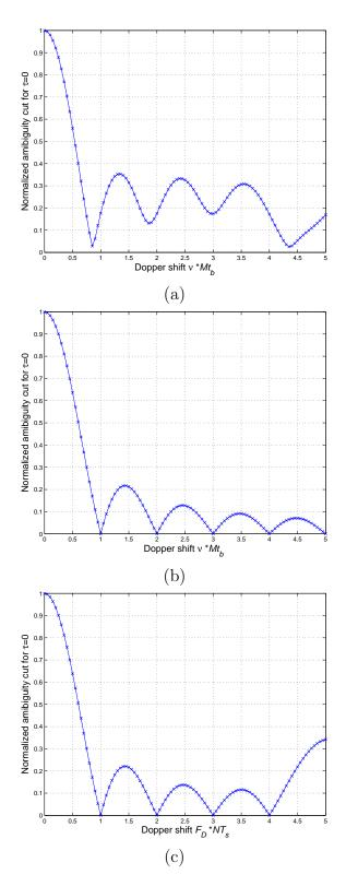
Figure 4.5. Doppler shift of codes(time delay=0): (a) 31-length Punctured binary sequence-pair (b) P4 code (c) 7x5-length Punctured binary sequence-pair.  $^{63}_{63}$
