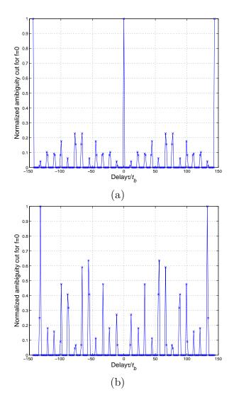
Figure 6.1. (a)Periodic autocorrelation property of 144-length optimized punctured ZCZ sequence-pair  $(x_1, y_1)$  (b)Periodic cross correlation property of 144-length optimized punctured ZCZ sequence-pair  $(x_1, y_2)$ .
