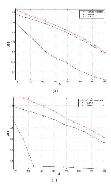
Figure 9.2. MSE versus M for fixed N=500 and SNR=20dB: (a)K=40; (b)K=100 .
