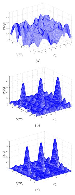
Figure 4.4. 3-D view of ambiguity function of sequence-pair: (a) M=1 (b) M=4 (c) M=10.  $$c_1$$
