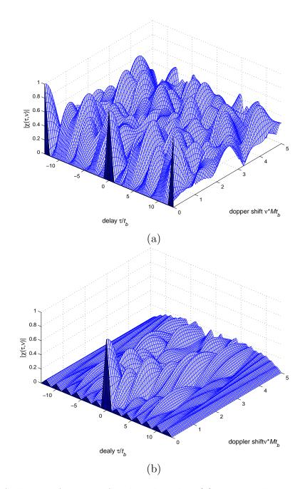
Figure 4.2. Ambiguity function of 13-length codes: (a) Punctured binary sequencepair (b) Barker code.
