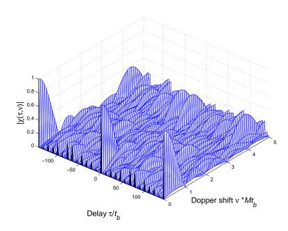
Figure 3.8. Ambiguity function of a 144-length ZCZ sequence-pair  $(x_i, y_i)$ .
