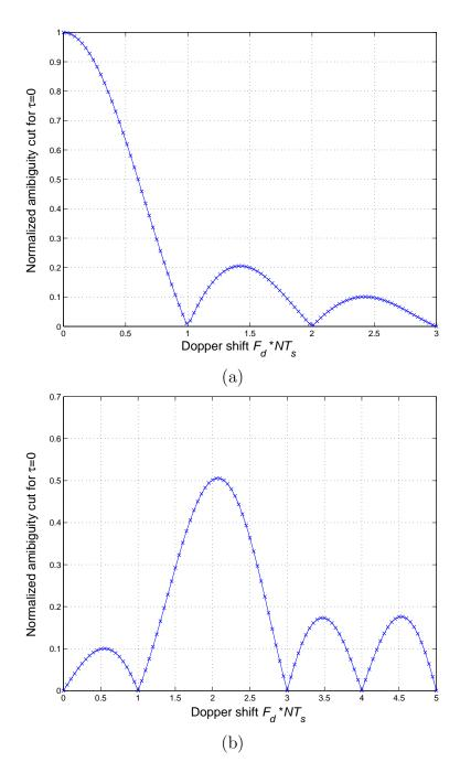
Figure 3.3. Doppler shift of 124-length ZCZPS(time delay=0): (a) autocorrelation (b) cross correlation.
