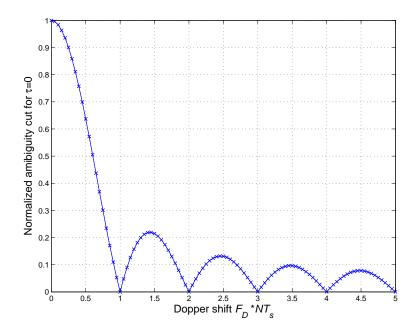
Figure 3.6. Doppler shift performance of 84-length LCZPS (time delay=0): autocorrelation.
