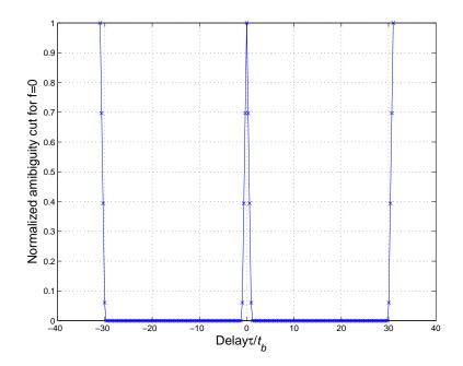
Figure 4.1. Periodic autocorrelation property of 31-length punctured binary sequencepair.
