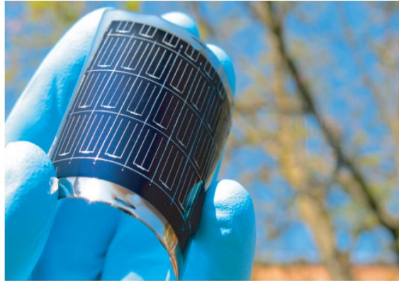
Fig. 1.17 The 18.7% efficiency of CIGS on PI films [28].
