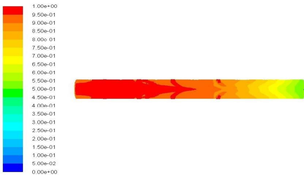
Figure 3.32 Contour plot of methane/air mixture is same configuration as Case 2 but with the openings replaced by "showerheads" at 30 ms
