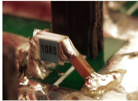
Figure 5.4. RC snubber implementation.
