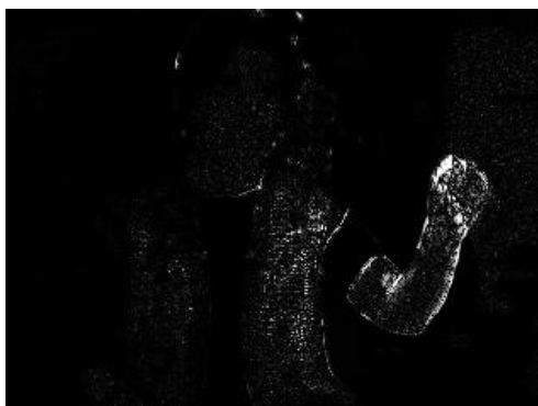
Figure 4.4 – Skin-motion image. The figure shows image obtained after pixel-wise multiplication of the skin likelihood score image and motion score image for the frame shown in figure 4.1.
