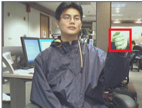
Figure 4.7 – Hand detection in model sequences with user wearing colored gloves and using full sleeved shirt.
