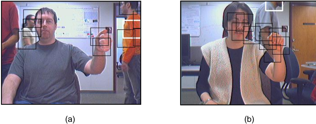
Figure 1.1 - Illustrates that the low level hand detection can often fail to provide perfect hand detection in presence of moving skin colored distractors. In the examples (a) and (b), the skin color and motion were collectively used to identify hand candidates. The hand candidate marked with white rectangle is the top detection result which is not the correct one.
