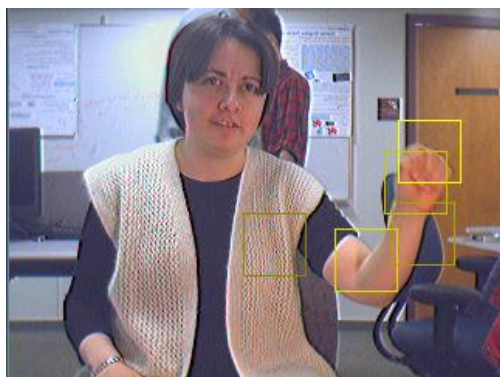
Figure 4.6 – Displays top five hand candidates detected from the input video sequence frame shown in figure 4.1
