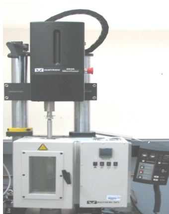
Figure 8.2 Instron MicroTester® used for shear and fiber pull tests.
