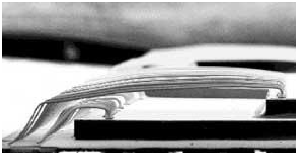
Figure 2.9 Forward ball bonding loops in stacked die applications [57].
