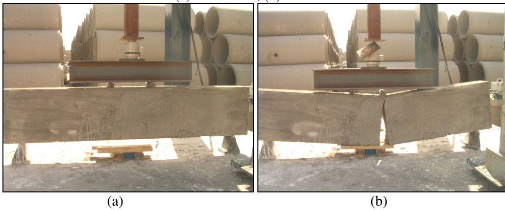
Figure B.15 Beam for concrete cast on 10/27/06 for 3 day test; (a) before test, (b) after test
