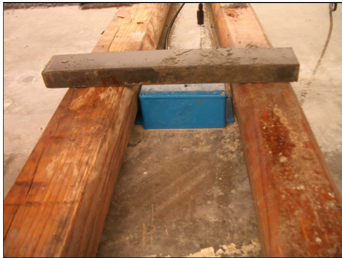
Figure 3.4 Displacement sensor attached to the middle under the beam with wooden protection after concrete beams were failed
