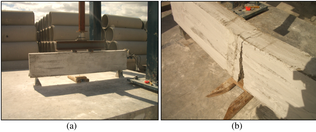
Figure B.11 Beam for 2 nd batch concrete cast on 10/26/06 for 1 day test; (a) before test, (b) after test
