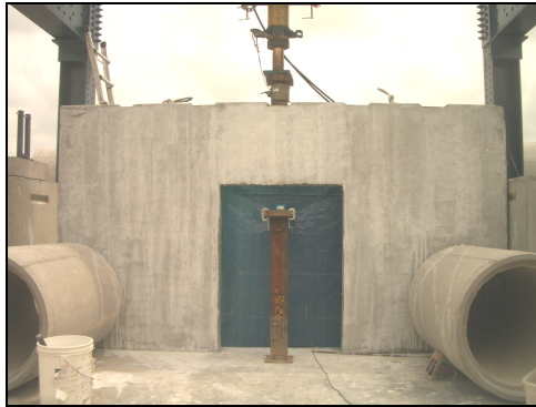
Figure C.13 Set up equipment for wall with door opening test
