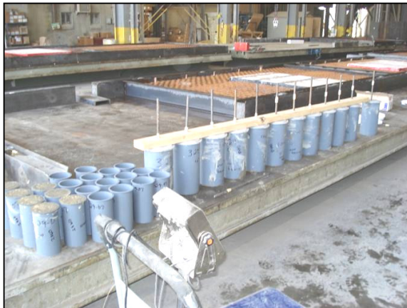
Figure A.18 Concrete specimens for pull-out test
