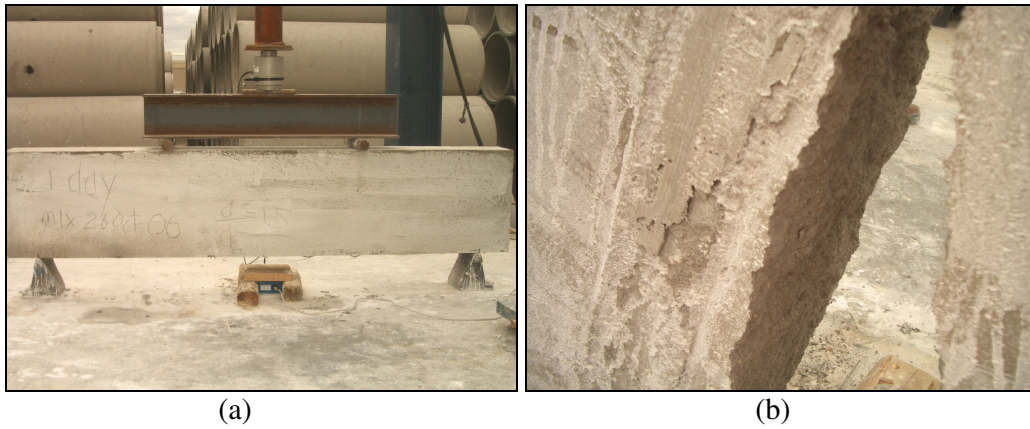
Figure B.6 Beam for 1 st batch concrete cast on 10/26/06 for 1 day test; (a) before test, (b) after test
