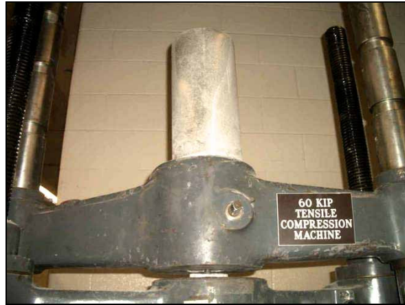
Figure 2.23 Pull-out test with universal material testing machine
