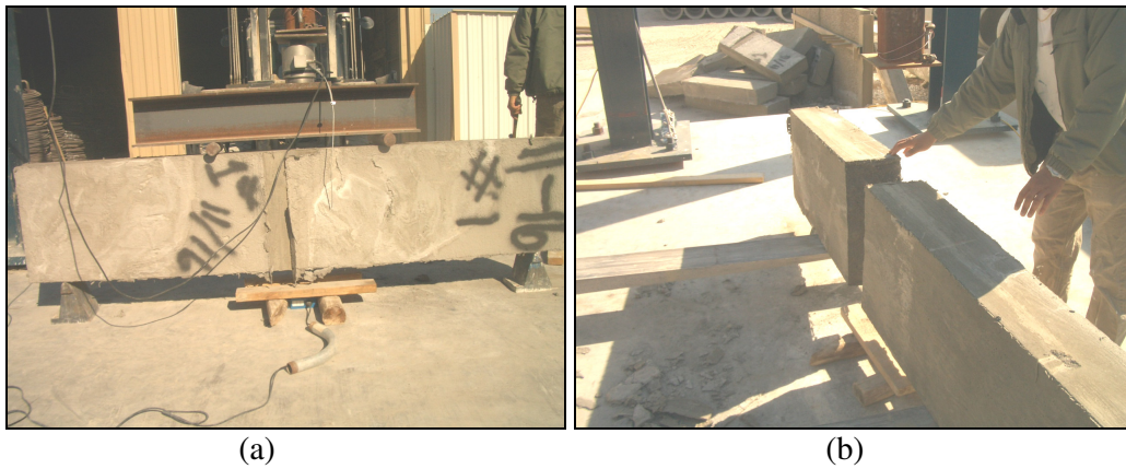
Figure B.41 Beam for 1 st batch concrete cast on 11/16/06 for 3 day test; (a) before test, (b) after test
