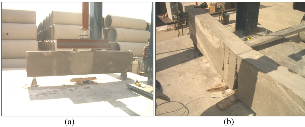
Figure B.18 Beam for 1 st batch concrete for concrete cast on 10/31/06 for 3 day test; (a) before test, (b) after test
