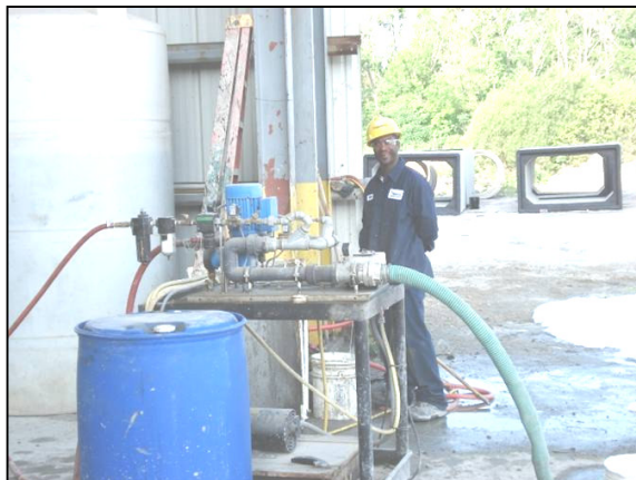
Figure A.3 Machine for mixing foaming agent
