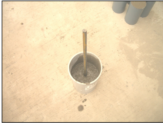
Figure A.16 Concrete specimens for pull-out test
