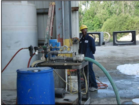
Figure 2.4 Mixing machine used for foaming agent
