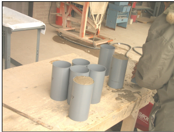
Figure A.14 Pouring concrete for test specimens
