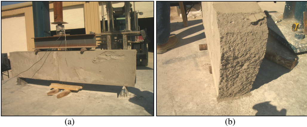
Figure B.23 Beam for 1 st batch concrete cast on 11/2/06 for 1 day test; (a) before test, (b) after test
