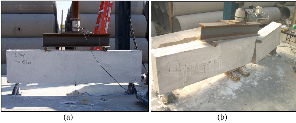
Figure B.1 Beam cast on 10/18/06 for 1 day test; (a) before test, (b) after test
