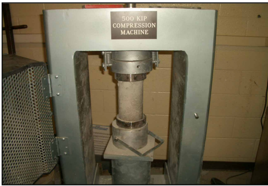
Figure 2.7 Compression machine for compressive strength test
