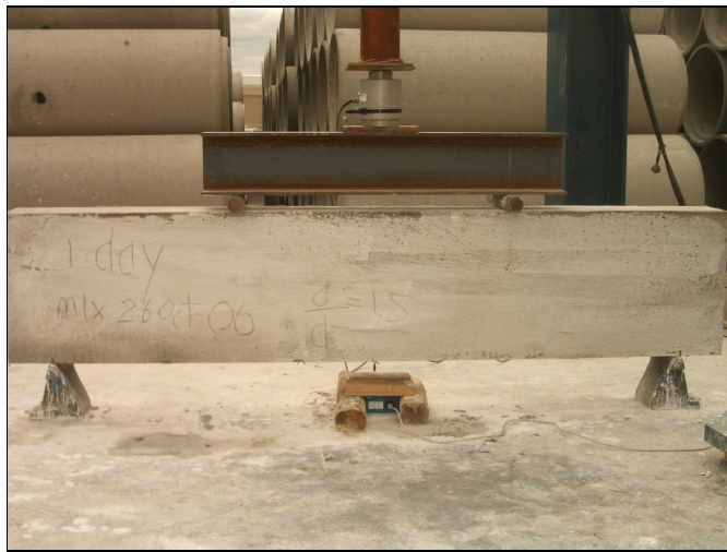
Figure 3.6 Set up position for loading and displacement sensor
