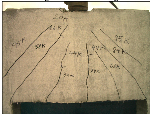
Figure C.19 Found another 45 degree crack at the right corner of opening at 84 kips
