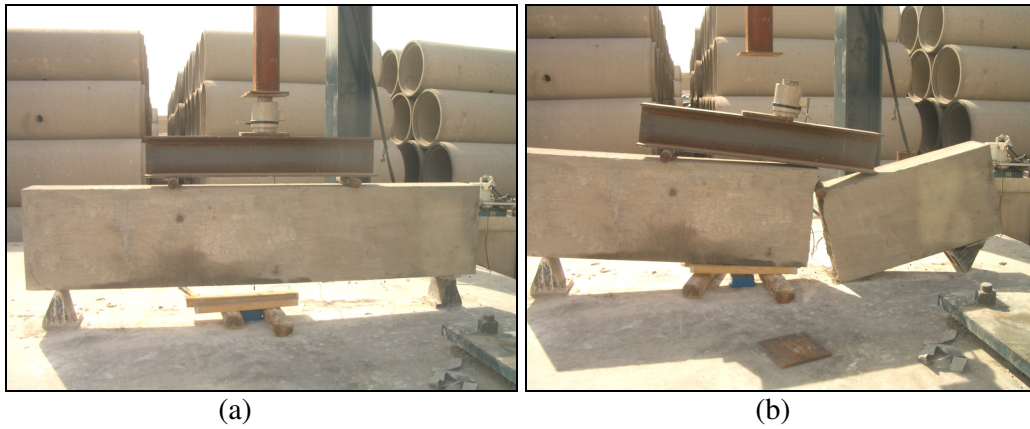
Figure B.19 Beam for 2 nd batch concrete cast on 10/31/06 for 3 day test; (a) before test, (b) after test
