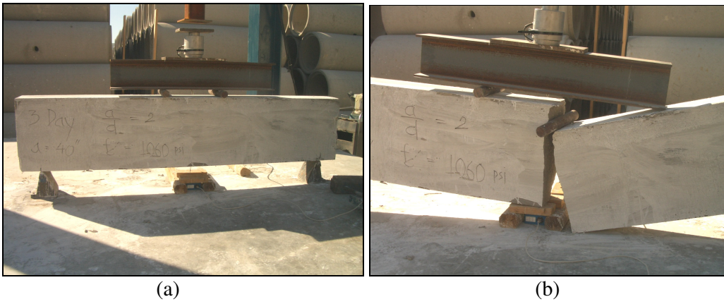
Figure B.2 Beam cast on 10/18/06 for 3 day test; (a) before test, (b) after test
