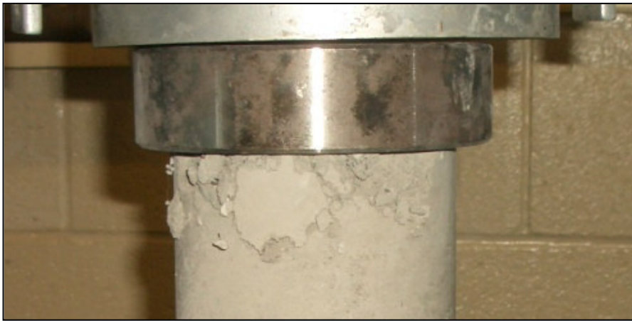
Figure 2.8 Failure of specimens for compressive test
