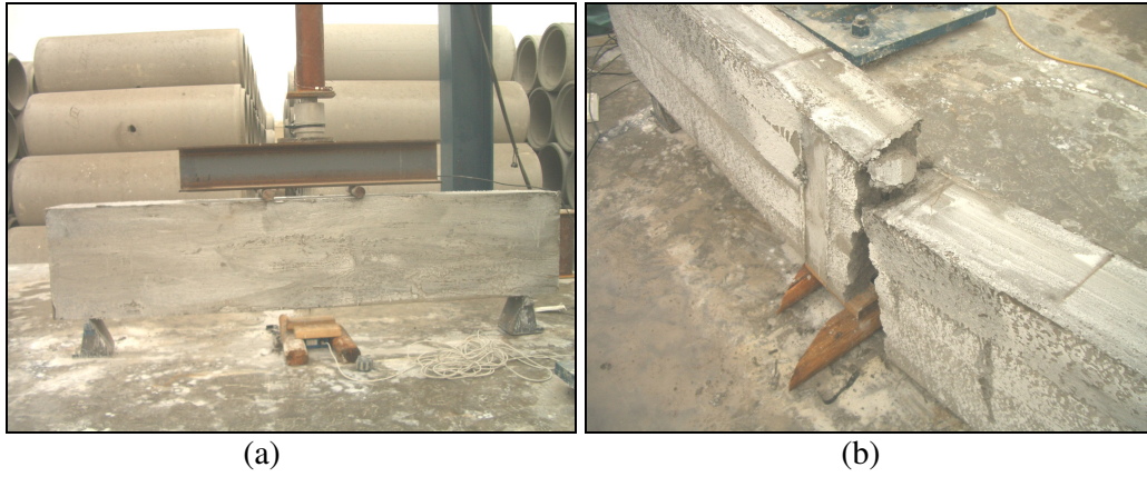
Figure B.4 Beam cast on 10/24/06 for 1 day test; (a) before test, (b) after test
