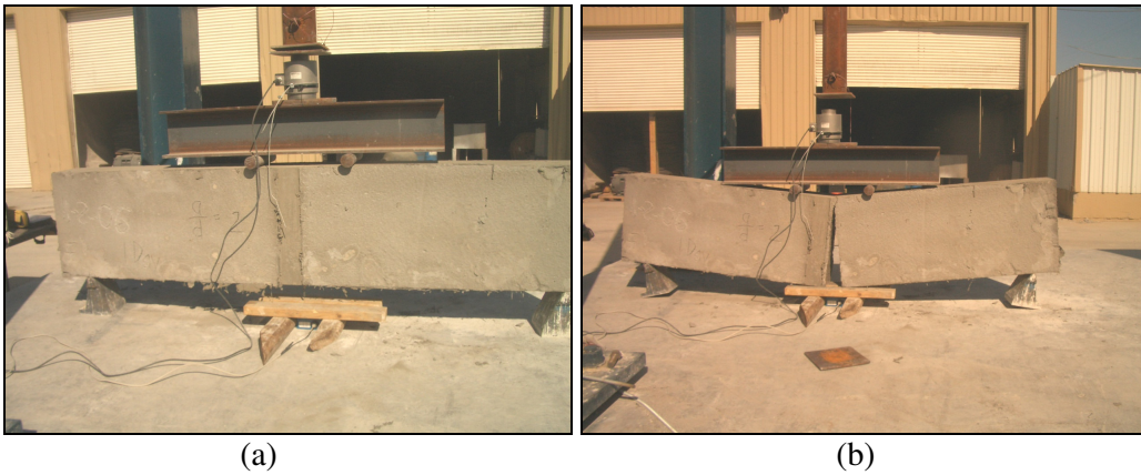
Figure B.24 Beam for 1 st batch concrete cast on 11/2/06 for 1 day test; (a) before test, (b) after test
