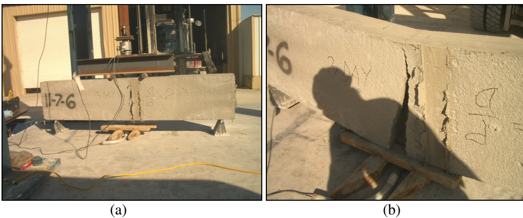
Figure B.33 Beam cast on 11/7/06 for 3 day test; (a) before test, (b) after test
