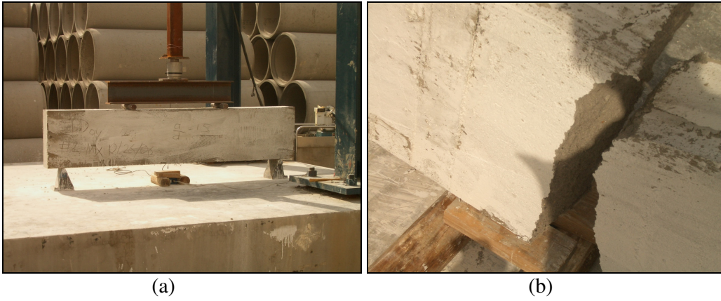
Figure B.10 Beam for 2 nd batch concrete cast on 10/26/06 for 1 day test; (a) before test, (b) after test
