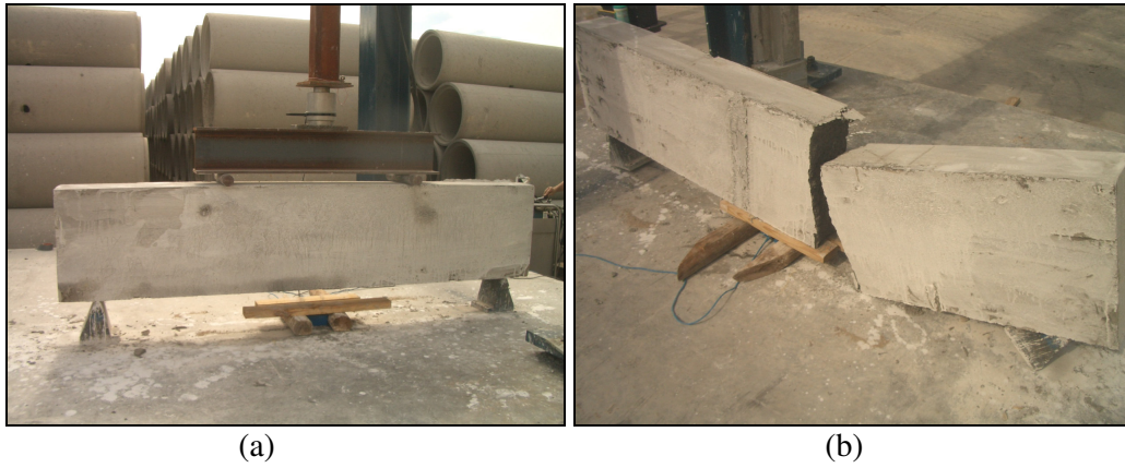
Figure B.14 Beam for concrete cast on 10/27/06 for 3 day test; (a) before test, (b) after test
