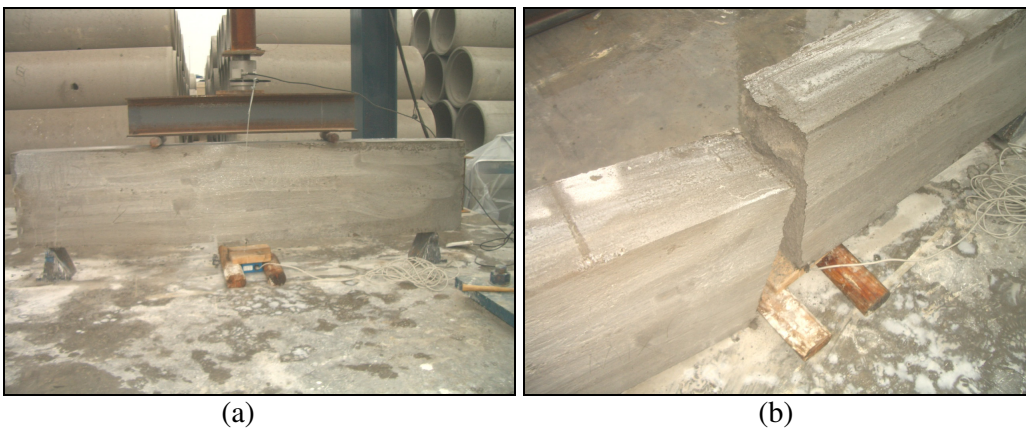
Figure B.3 Beam cast on 10/24/06 for 1 day test; (a) before test, (b) after test
