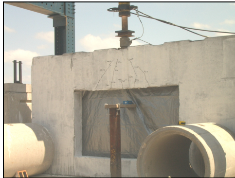
Figure C.9 Wall lost stiffness at 50 kips
