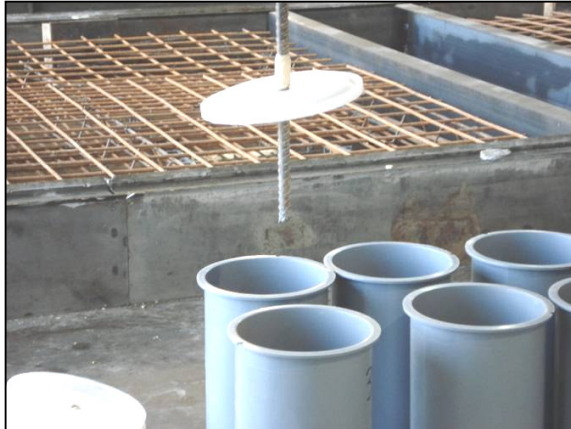
Figure A.17 Concrete specimens for pull-out test
