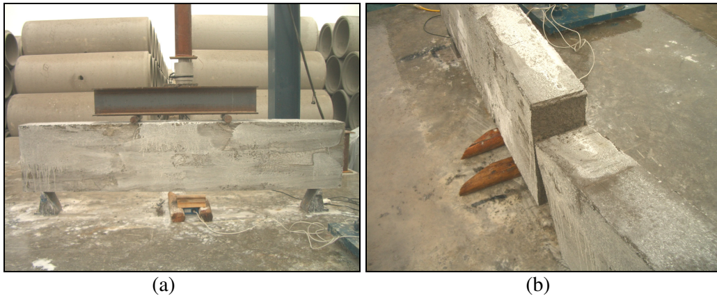
Figure B.5 Beam cast on 10/24/06 for 1 day test; (a) before test, (b) after test
