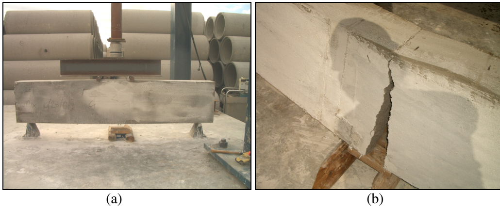
Figure B.7 Beam for 1 st batch concrete cast on 10/26/06 for 1 day test; (a) before test, (b) after test
