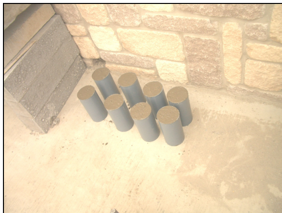
Figure A.15 Concrete specimens for compressive test
