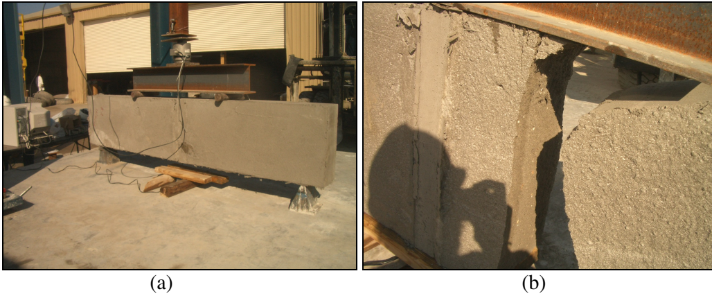
Figure B.22 Beam for 2 nd batch concrete cast on 10/31/06 for 7 day test; (a) before test, (b) after test
