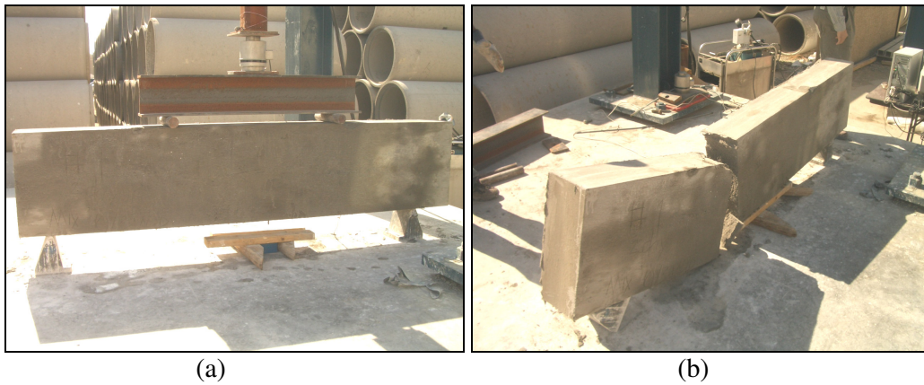
Figure B.17 Beam for 1 st batch concrete for concrete cast on 10/31/06 for 3 day test; (a) before test, (b) after test
