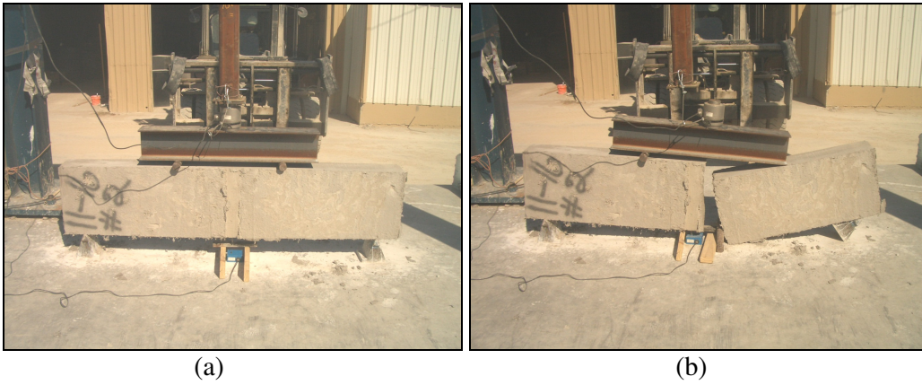
Figure B.53 Beam for 2 nd batch concrete cast on 11/16/06 for 90 day test; (a) before test, (b) after test
