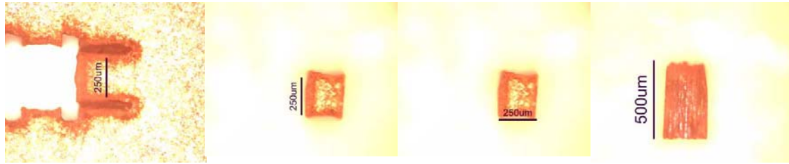
Figure 5.12 Machining on 55% porous copper layer used in assembly assisted by agitation.
