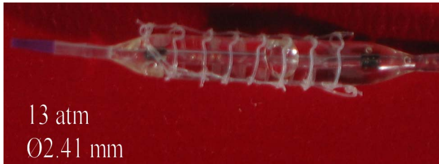
Fig. 3.14 Balloon with Stent Expansion at 13(atm)
