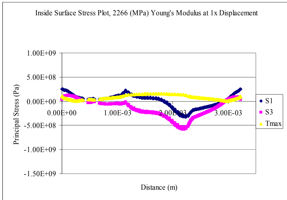
Fig. B.4 Inside Surface Principal Stress S1, S3, and Tmax for 2266(MPa)
