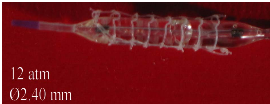
Fig. 3.13 Balloon with Stent Expansion at 12(atm)
