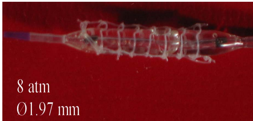
Fig. 3.9 Balloon with Stent Expansion at 8(atm)
