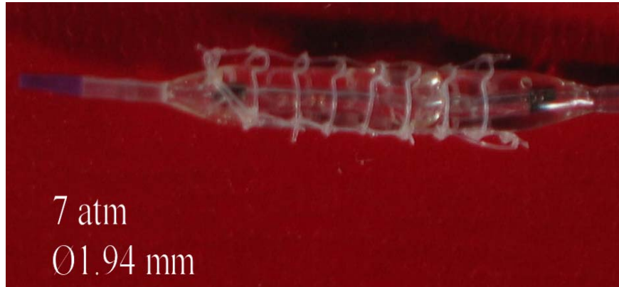
Fig. 3.8 Balloon with Stent Expansion at 7(atm)
