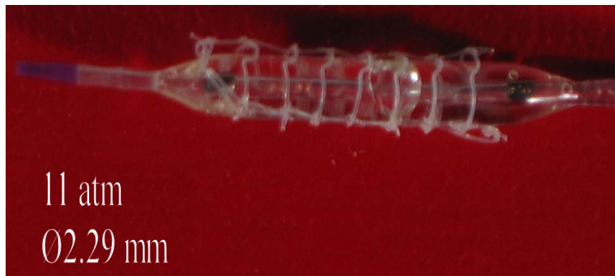
Fig. 3.12 Balloon with Stent Expansion at 11(atm)
