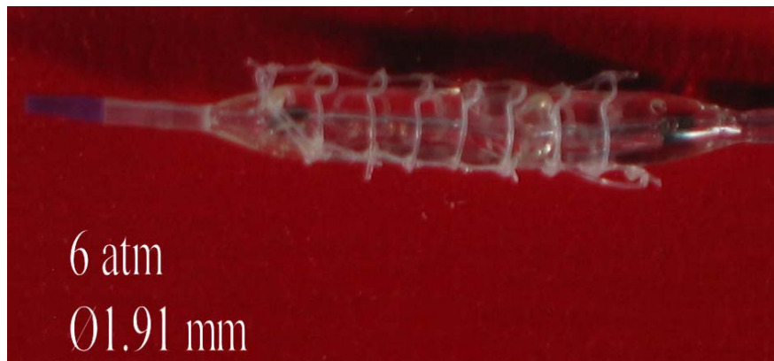
Fig. 3.7 Balloon with Stent Expansion at 6(atm)
