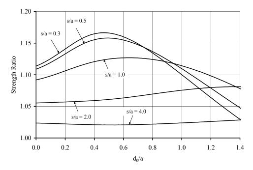
Figure F.5 Two hole strength prediction for (0/100/0) laminate, equal holes. Holes oriented in-line with the load. Low s/a values.
