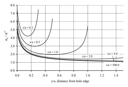
Figure E.1 Stress profile for (50/0/50) laminate, equal holes. Holes oriented transverse to the load.
