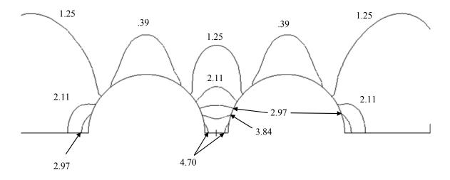
Figure D.3 Contour plot of *x*-component of stress for quasi-isotropic laminate with equal holes.
