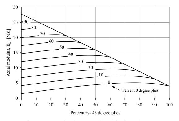
Figure 3.1 Carpet plot of apparent axial modulus for IM7/977-3.
