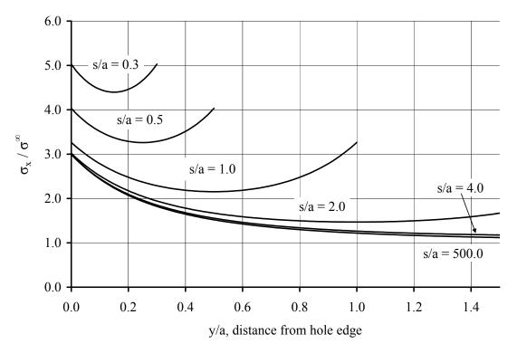
Figure 5.9 Stress profile for (25/50/25) laminate, equal holes. Holes oriented transverse to the load.
