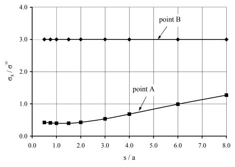
Figure 5.8 Stress concentration for two holes, b/a = 10.0. (25/50/25) laminate, holes oriented in-line with the load.
