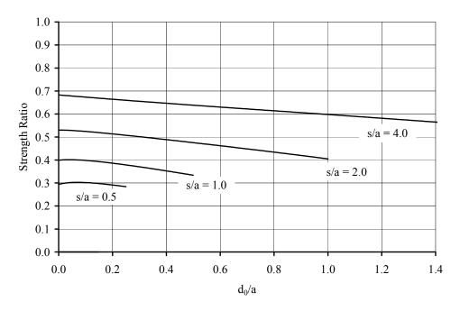
Figure F.2 Two hole strength prediction for (50/0/50) laminate, b/a = 10.0. Holes oriented transverse to the load.
