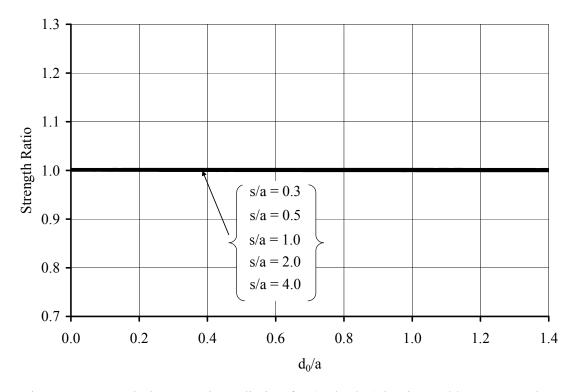
Figure 5.22 Two hole strength prediction for (25/50/25) laminate, b/a = 5.0. Holes oriented in-line with the load.
