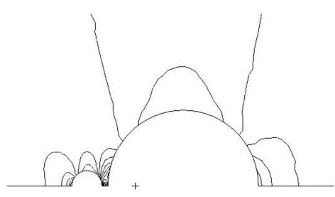
Figure D.6 Overview contour plot of *x*-component of stress for quasi-isotropic laminate with unequal holes.
