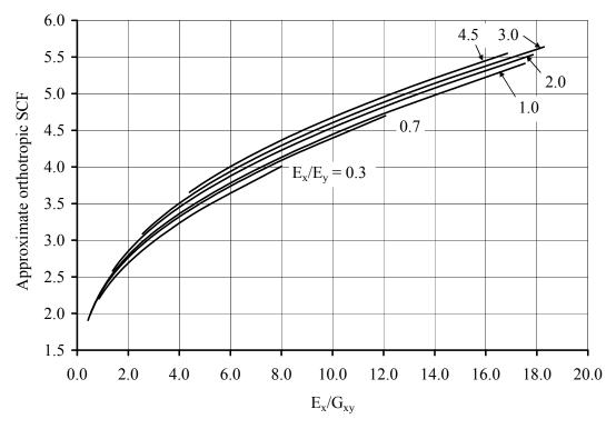
Figure 3.5 Approximate orthotropic stress concentration factor.
