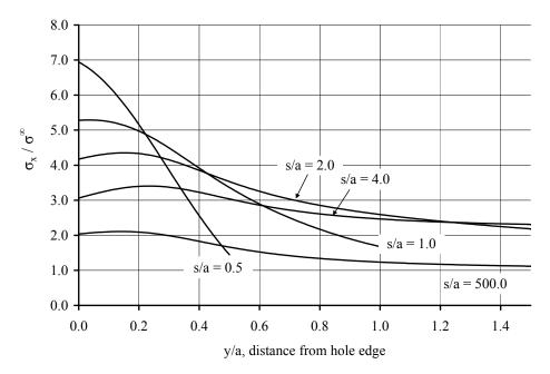
Figure E.15 Stress profile for (0/100/0) laminate, b/a = 10.0. Holes oriented transverse to the load.
