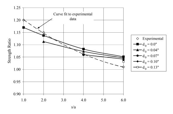
Figure 5.26 Comparison of strength prediction method to experimental data for holes oriented in-line with the load.
