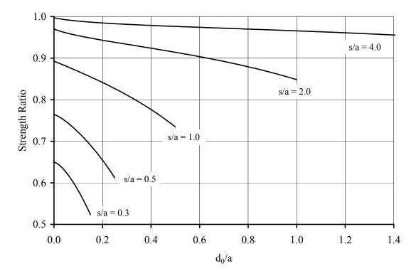
Figure 5.14 Two hole strength prediction for (50/0/50) laminate, equal holes. Holes oriented transverse to the load.
