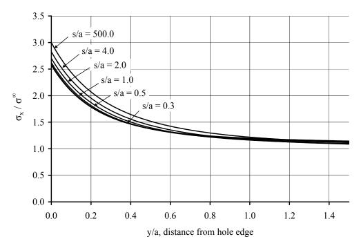
Figure 5.11 Stress profile for (25/50/25) laminate, equal holes. Holes oriented in-line with the load.
