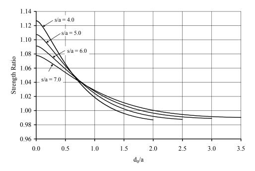
Figure F.7 Two hole strength prediction for (50/0/50) laminate, equal holes. Holes oriented in-line with the load. High s/a values.
