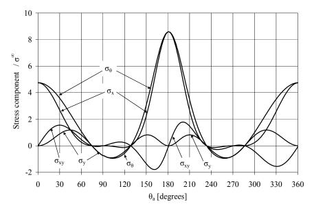
Figure H.2 Stress components at smaller hole edge for (25/50/25) laminate, b/a = 5.0, s/a = 0.5. Holes oriented transverse to the load.
