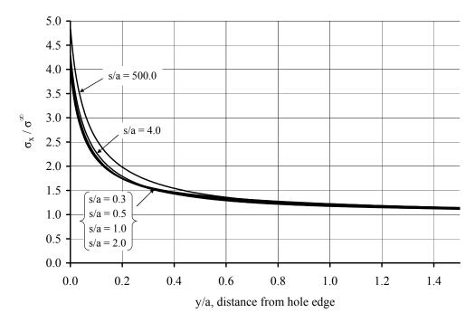
Figure E.17 Stress profile for (50/0/50) laminate, equal holes. Holes oriented in-line with the load.
