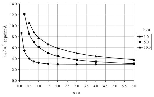
Figure 5.6 Stress concentration for various hole size ratios. (25/50/25) laminate, holes oriented transverse to the load.
