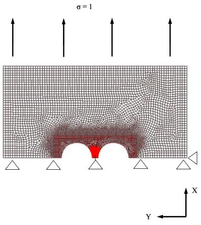
Figure D.1 Finite element model with equal holes.
