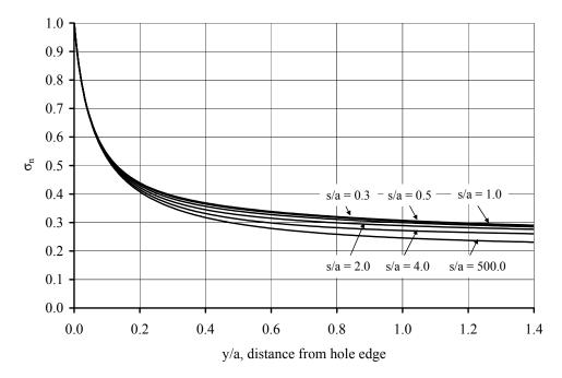
Figure E.18 Normalized stress profile for (50/0/50) laminate, equal holes. Holes oriented in-line with the load.
