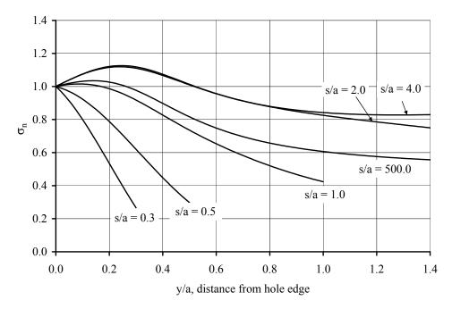
Figure E.10 Normalized stress profile for (0/100/0) laminate, b/a = 5.0. Holes oriented transverse to the load.
