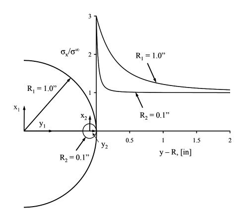
Figure 2.3 Stress profiles for two different sized holes in a uniaxally loaded, isotropic material.
