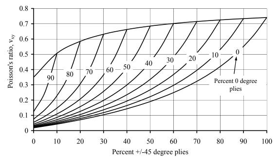
Figure 3.3 Carpet plot of apparent Poisson's ratio for IM7/977-3.
