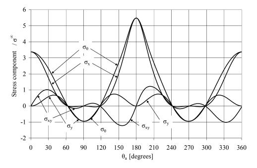
Figure H.1 Stress components at hole edge for (25/50/25) laminate, equal holes, s/a = 0.25. Holes oriented transverse to the load.
