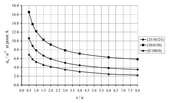
Figure 5.5 Stress concentration for two holes, b/a = 10.0. Holes oriented transverse to the load.
