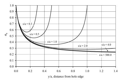
Figure E.2 Normalized stress profile for (50/0/50) laminate, equal holes. Holes oriented transverse to the load.
