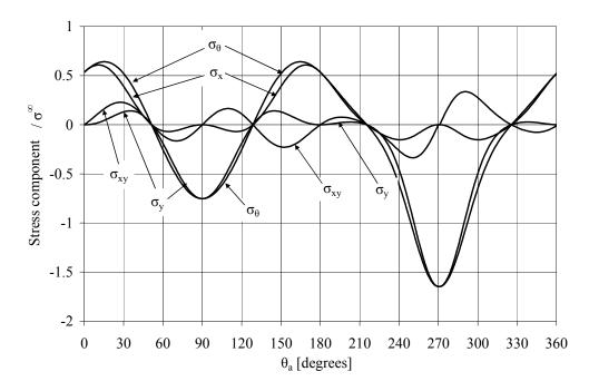
Figure H.5 Stress components at smaller hole edge for (25/50/25) laminate, b/a = 5.0, s/a = 0.5. Holes oriented in-line with the load.
