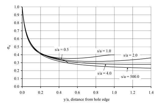
Figure E.14 Normalized stress profile for (50/0/50) laminate, b/a = 10.0. Holes oriented transverse to the load.
