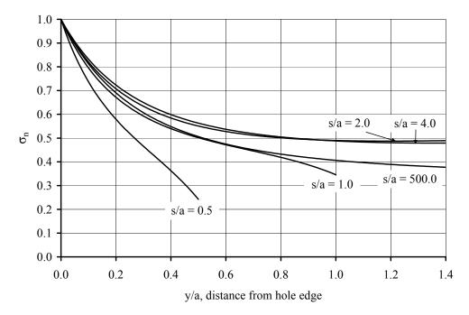
Figure E.12 Normalized stress profile for (25/50/25) laminate, b/a = 10.0. Holes oriented transverse to the load.
