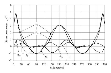
Figure H.3 Stress components at larger hole edge for (25/50/25) laminate, b/a = 5.0, s/a = 0.5. Holes oriented transverse to the load.
