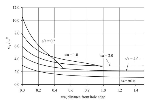
Figure E.11 Stress profile for (25/50/20) laminate, b/a = 10.0. Holes oriented transverse to the load.
