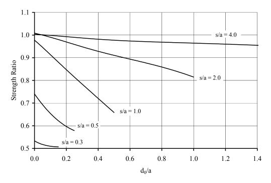
Figure 5.15 Two hole strength prediction for (0/100/0) laminate, equal holes. Holes oriented transverse to the load.
