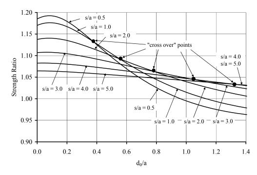
Figure 5.25 Two hole strength prediction for T800/924C, (50/50/0) laminate. Holes oriented in-line with the load.
