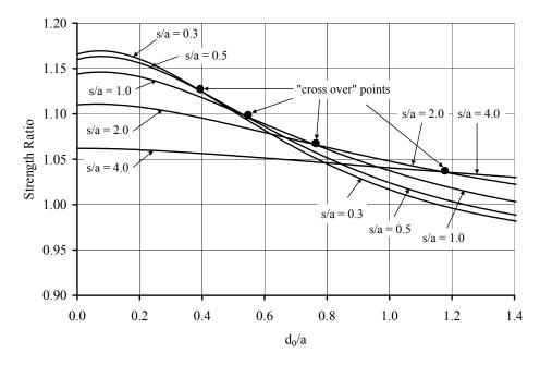
Figure 5.21 Two hole strength prediction for (25/50/25) laminate, equal holes. Holes oriented in-line with the load. Low s/a values.
