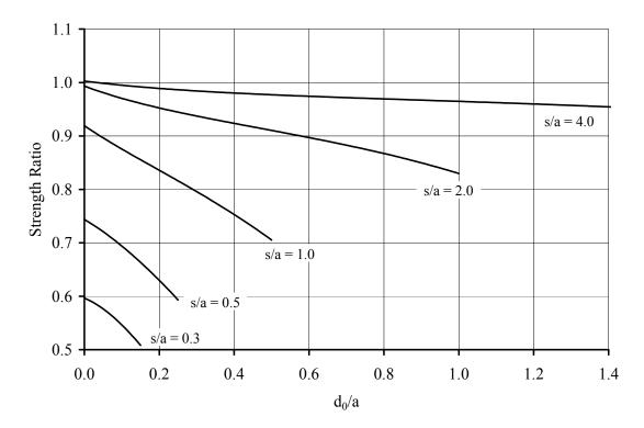
Figure 5.13 Two hole strength prediction for (25/50/25) laminate, equal holes. Holes oriented transverse to the load.
