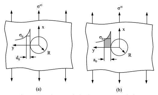
Figure 2.4 (a) Point stress criterion (b) Average stress criterion.
