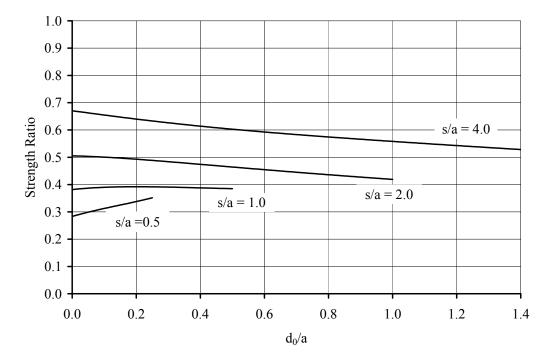
Figure F.1 Two hole strength prediction for (25/50/25) laminate, b/a = 10.0. Holes oriented transverse to the load.
