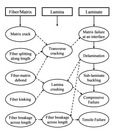
Figure 2.2 Various failure modes at different scales.
