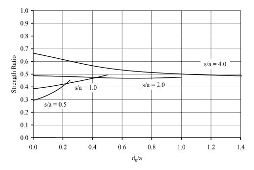
Figure F.3 Two hole strength prediction for (0/100/0) laminate, b/a = 10.0. Holes oriented transverse to the load.
