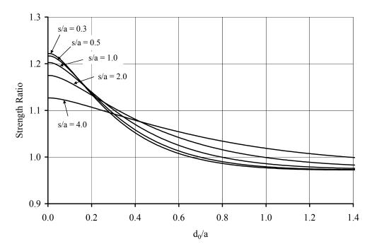
Figure F.4 Two hole strength prediction for (50/0/50) laminate, equal holes. Holes oriented in-line with the load. Low s/a values.
