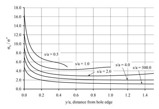
Figure E.13 Stress profile for (50/0/50) laminate, b/a = 10.0. Holes oriented transverse to the load.
