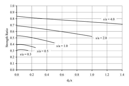
Figure 5.19 Two hole strength prediction for (50/0/50) laminate, b/a = 5.0. Holes oriented transverse to the load.
