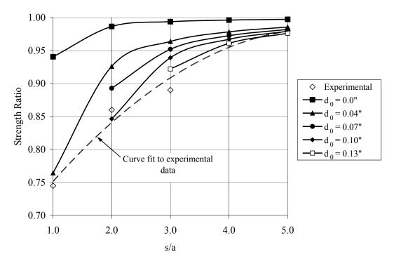
Figure 5.24 Comparison of strength prediction method to experimental data for holes oriented transverse to the load.
