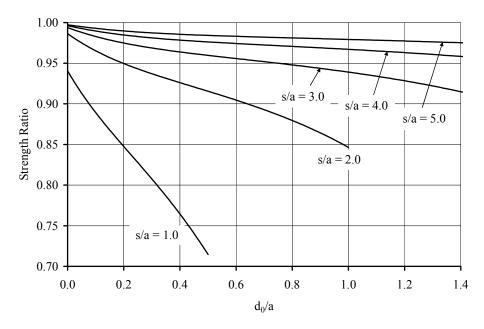
Figure 5.23 Two hole strength prediction for T800/924C, (50/50/0) laminate. Holes oriented transverse to the load.
