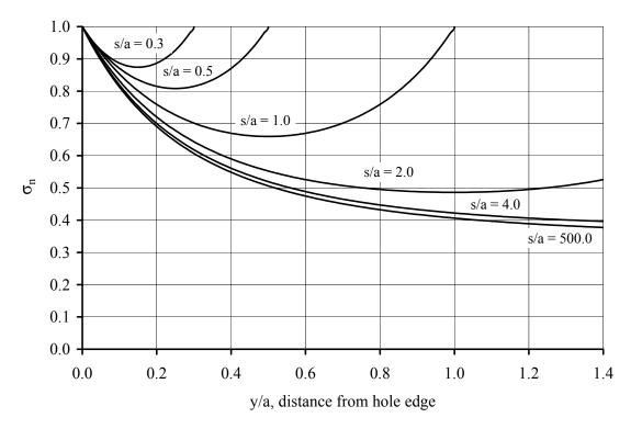
Figure 5.10 Normalized stress profile for (25/50/25) laminate, equal holes. Holes oriented transverse to the load.
