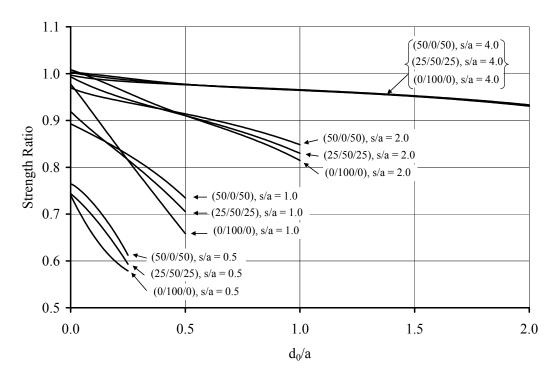
Figure 5.16 Two hole strength prediction for three laminates, equal holes. Holes oriented transverse to the load. Low s/a values.
