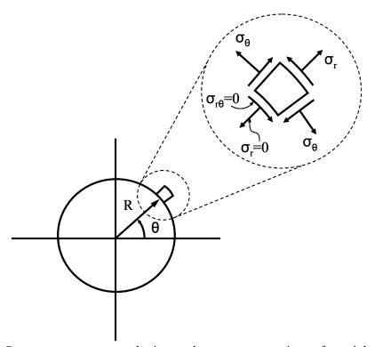
Figure 4.1 Stress components on the internal contour.  $\sigma_{\theta}$  – circumferential stress,  $\sigma_r$  – radial stress,  $\sigma_{r\theta}$  – tangential shear stress.
