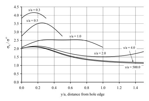
Figure E.3 Stress profile for (0/100/0) laminate, equal holes. Holes oriented transverse to the load.
