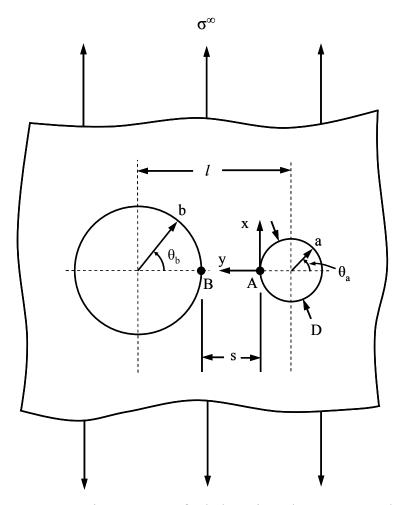
Figure 5.1 Geometric parameters for holes oriented transverse to the load.
