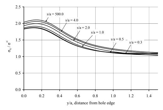
Figure E.19 Stress profile for (0/100/0) laminate, equal holes. Holes oriented in-line with the load.
