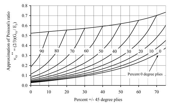
Figure 3.7 Approximation of Poisson's ratio for IM7/977-3 where  $v_{xy}^{**} = C_I G_{xy}/E_y = (2/3)(G_{xy}/E_y).$
