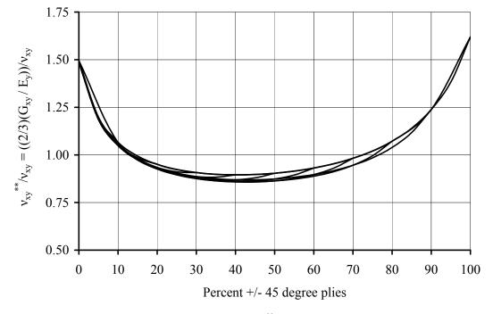
Figure 3.8 Carpet plot of  $v_{xy}^{**}/v_{xy}$  for IM7/977-3.
