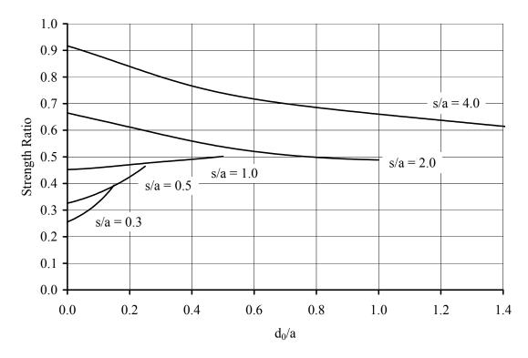
Figure 5.20 Two hole strength prediction for (0/100/0) laminate, b/a = 5.0. Holes oriented transverse to the load.
