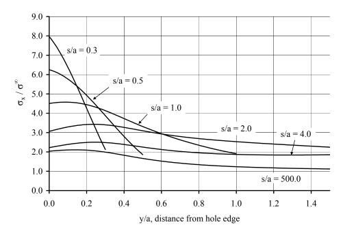
Figure E.9 Stress profile for (0/100/0) laminate, b/a = 5.0. Holes oriented transverse to the load.
