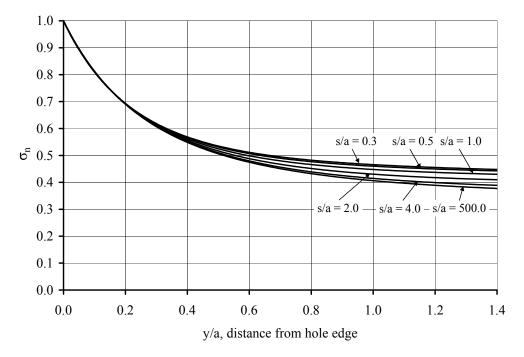
Figure 5.12 Normalized stress profile for (25/50/25) laminate, equal holes. Holes oriented in-line with the load.
