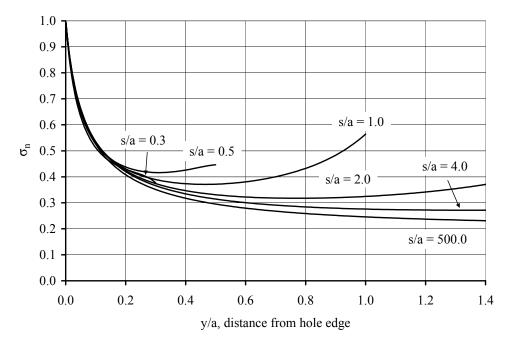
Figure E.8 Normalized stress profile for (50/0/50) laminate, b/a = 5.0. Holes oriented transverse to the load.
