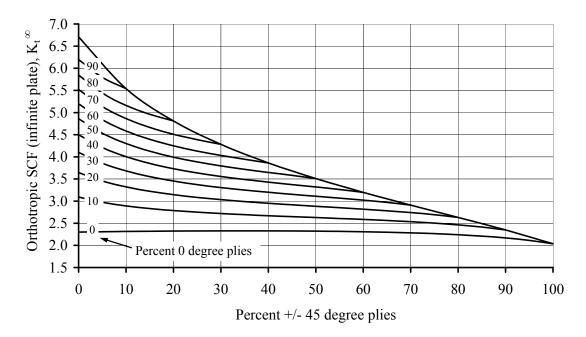
Figure 3.4 Carpet plot of apparent orthotropic stress concentration factor for IM7/977-3.
