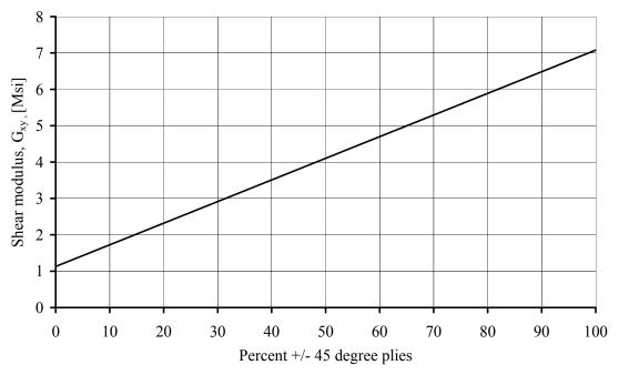
Figure 3.2 Carpet plot of apparent shear modulus for IM7/977-3.
