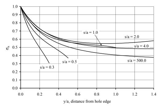
Figure E.6 Normalized stress profile for (25/50/25) laminate, b/a = 5.0. Holes oriented transverse to the load.
