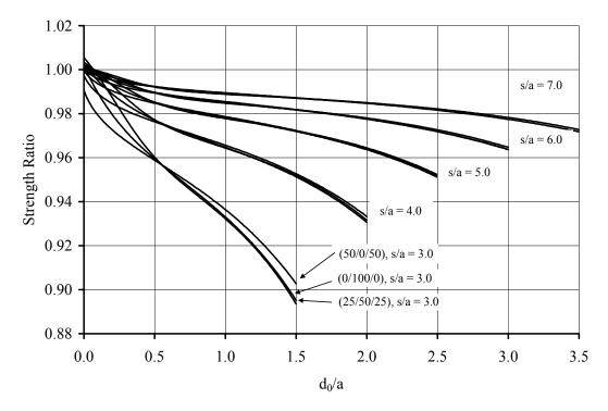
Figure 5.17 Two hole strength prediction for three laminates, equal holes. Holes oriented transverse to the load. High s/a values.
