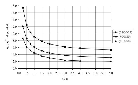
Figure 5.4 Stress concentration for two holes, b/a = 5.0. Holes oriented transverse to the load.
