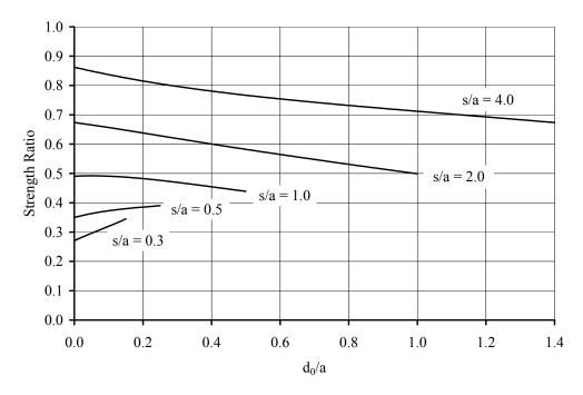
Figure 5.18 Two hole strength prediction for (25/50/25) laminate, b/a = 5.0. Holes oriented transverse to the load.
