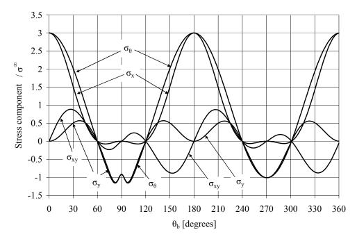
Figure H.6 Stress components at larger hole edge for (25/50/25) laminate, b/a = 5.0, s/a = 0.5. Holes oriented in-line with the load.
