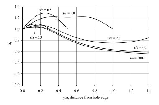
Figure E.4 Normalized stress profile for (0/100/0) laminate, equal holes. Holes oriented transverse to the load.
