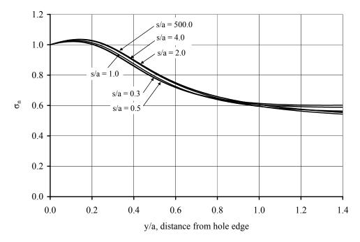
Figure E.20 Normalized stress profile for (0/100/0) laminate, equal holes. Holes oriented in-line with the load.
