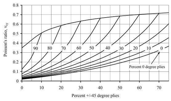
Figure 3.6 Exact value of Poisson's ratio for IM7/977-3.
