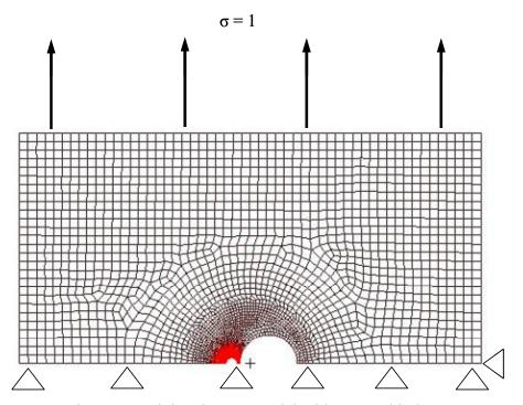
Figure D.4 Finite element model with unequal holes.
