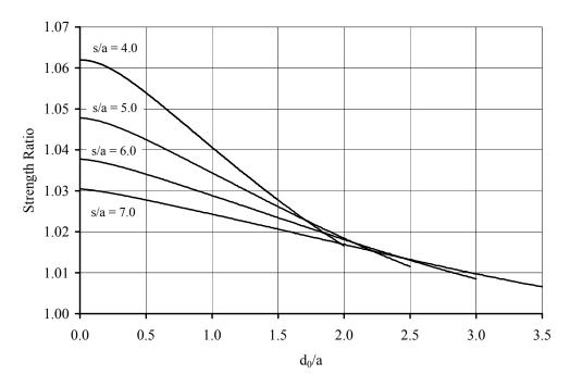
Figure F.6 Two hole strength prediction for (25/50/0) laminate, equal holes. Holes oriented in-line with the load. High s/a values.
