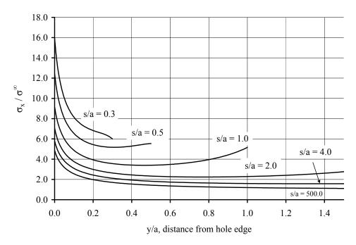
Figure E.7 Stress profile for (50/0/50) laminate, b/a = 5.0. Holes oriented transverse to the load.
