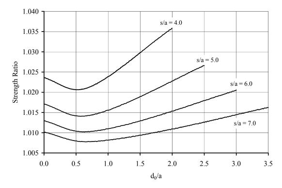
Figure F.8 Two hole strength prediction for (0/100/0) laminate, equal holes. Holes oriented in-line with the load. High s/a values.
