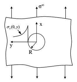
Figure 2.1 Stress profile for a uniaxially loaded plate with a circular hole.
