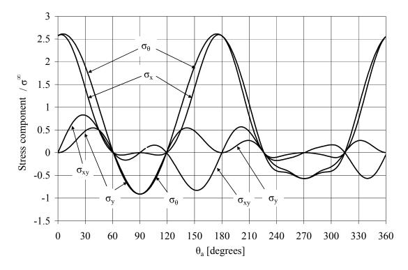
Figure H.4 Stress components at hole edge for (25/50/25) laminate, equal holes, s/a = 0.25. Holes oriented in-line with the load.
