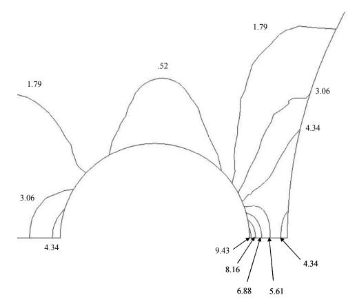
Figure D.7 Detail contour plot of *x*-component of stress for quasi-isotropic laminate with unequal holes.
