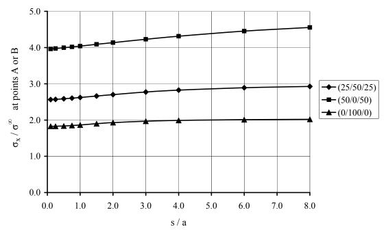
Figure 5.7 Stress concentration for two equal holes. Holes oriented in-line with the load.
