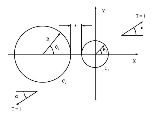
Figure C.2 Parameters for two unequal size holes for comparison to Haddon's solution.
