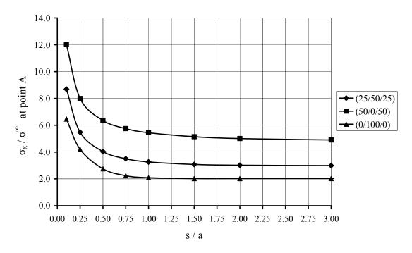
Figure 5.3 Stress concentration for two equal holes. Holes oriented transverse to the load.
