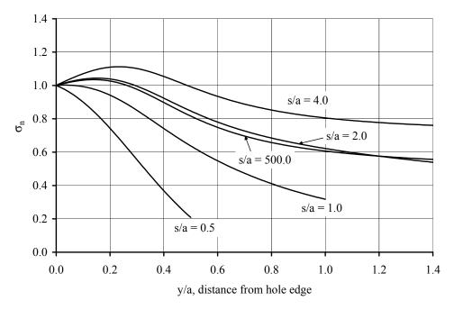
Figure E.16 Normalized stress profile for (0/100/0) laminate, b/a = 10.0. Holes oriented transverse to the load.
