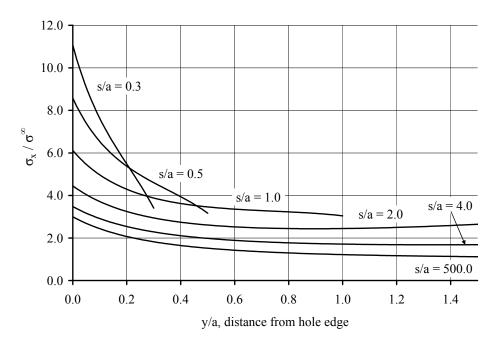
Figure E.5 Stress profile for (25/50/25) laminate, b/a = 5.0. Holes oriented transverse to the load.
