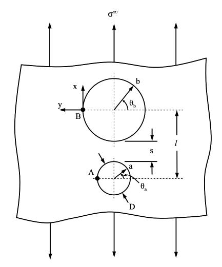
Figure 5.2 Geometric parameters for holes oriented in-line with the load.
