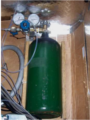
Figure 3.14 Zero gas cylinder for purging the OBS-1300 setup
