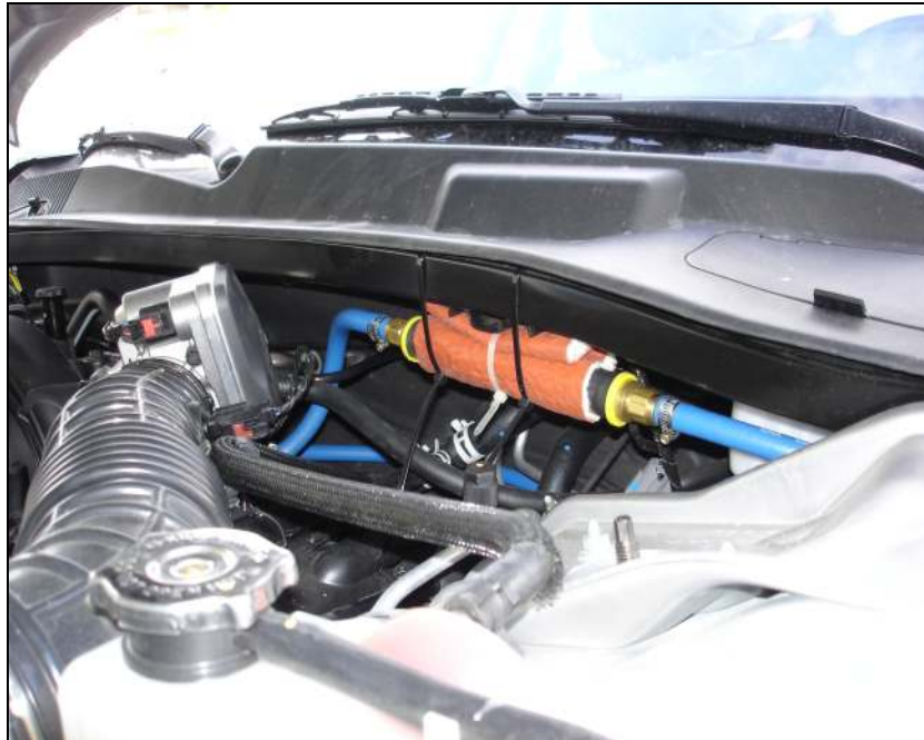
Figure 3.1 Installation of Clean Air Retrofit Device in the fuel line of the Dodge Charger 2007
