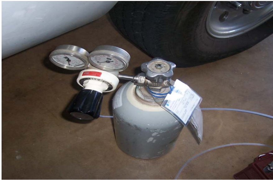
Figure 3.15 Calibration gas cylinder used in NO x sensor calibration
