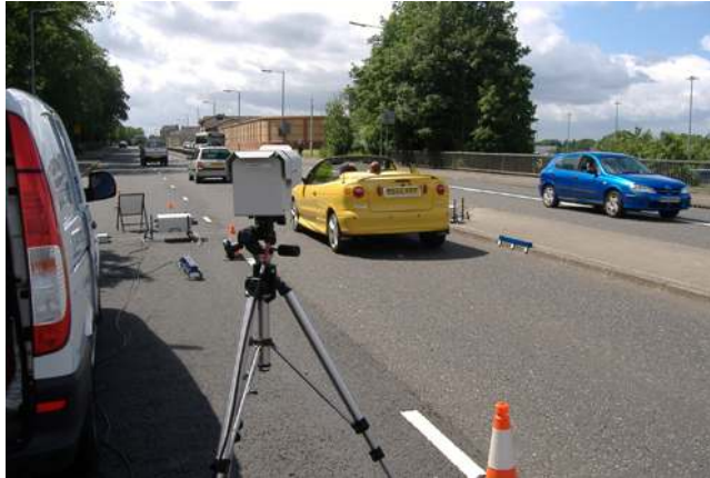
Figure 2.3 Vehicle emissions measurement by remote sensing ( http://www.et.co.uk/cgi-bin/products.cgi?section=1002&productcategory=1014 )
