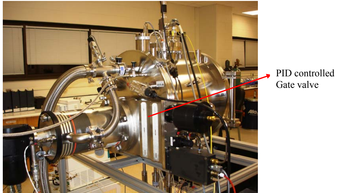
Figure 4.3 Side view of the hybrid plasma CVD and PVD system.
