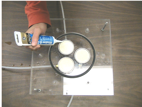
Figure 4.22 Bottom plate of custom-made chamber housing three 5-bar disks
