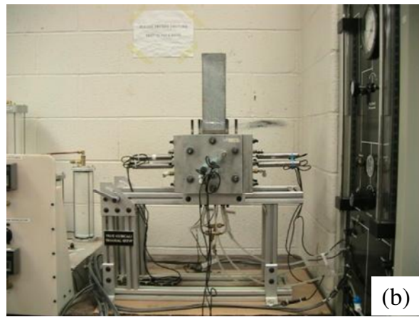
Figure 4.30 Lateral wall assemblies installation: (a) assembling process; (b) partially assembled cell with pluviation shaft
