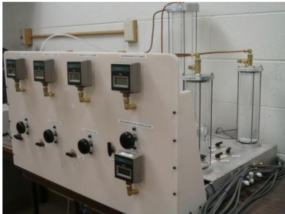
Figure 4.14 External pressure application panel
