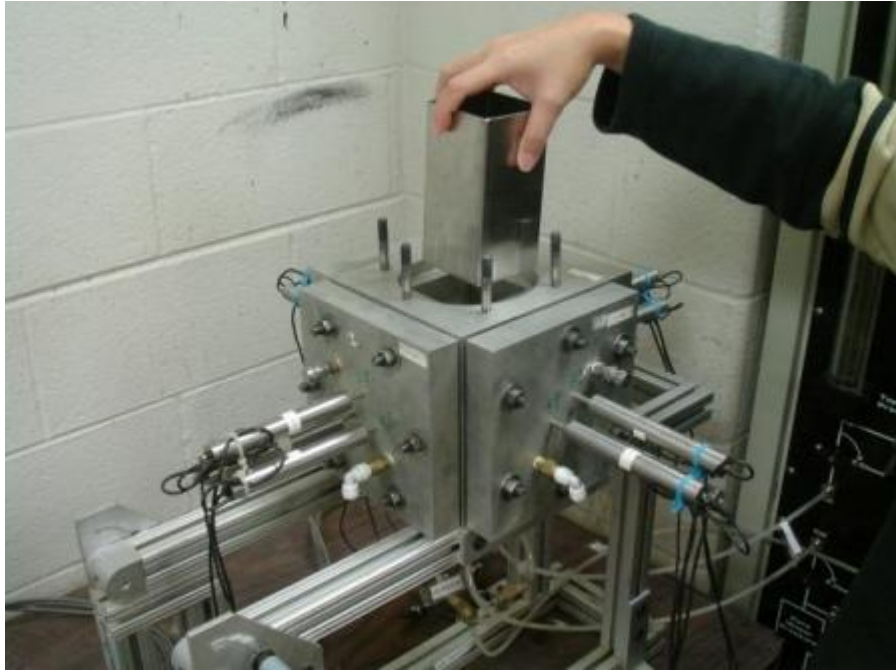
Figure 4.31 Removal of thin-walled pluviation shaft
