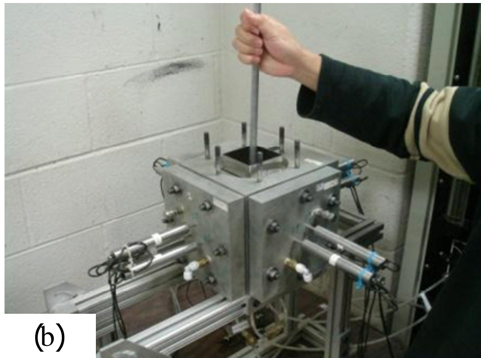
Figure 4.24 In-place combined pluviation and tamping compaction process: (a) pluviation process; (b) tamping compaction process
