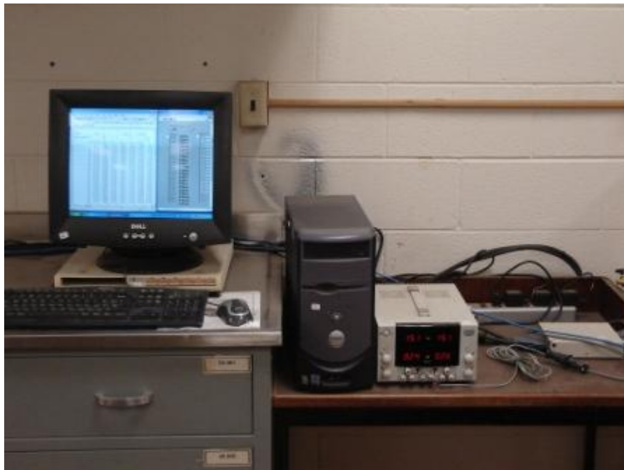
Figure 4.18 Photograph of soil pressure/deformation data acquisition system
