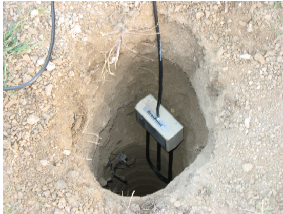
Figure 5.35 Field schematic of Gro-Point moisture probe installation
