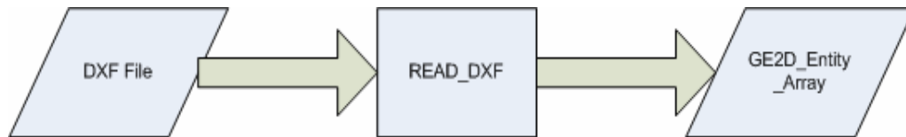
Figure 4.2: Read DXF File and store array of GE2D_Entity objects
