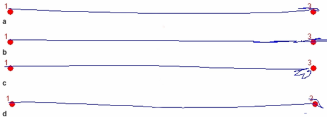
Figure 2.4 Average movements, from target 1 to 3 a) no effect b) spring effect c) damper effect d) ellipse effect
