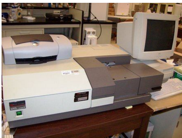
Figure 27: Perkin Elmer UV-Visible-NIR Spectroscopic unit.
