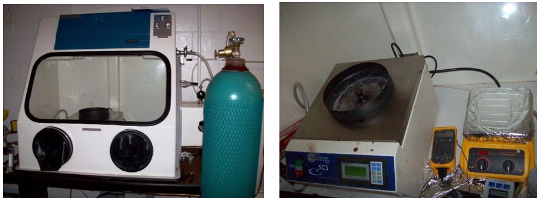
Figure 30: (a) Argon purged Glove box (b) Spin coater and hot plate
