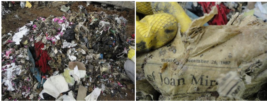
Figure 4.14 Partially Degraded Landfilled Samples
