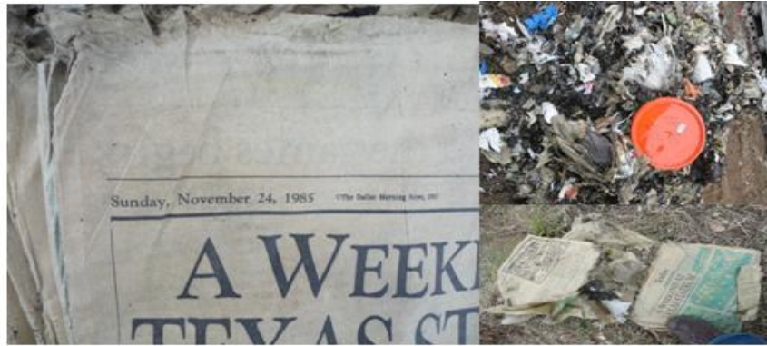
Figure 4.4 Partially-Degraded Samples from 40 ft, 50 ft and 60 ft Depth of Boring B-70
