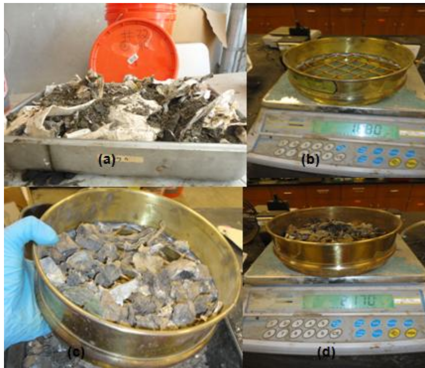
Figure 3.10 (a) Oven Dried Sample (b) Weighed Empty Sieve (c) Retaining Samples on the Sieve (d) Weight of the Sieve with the Sample Retaining on It
