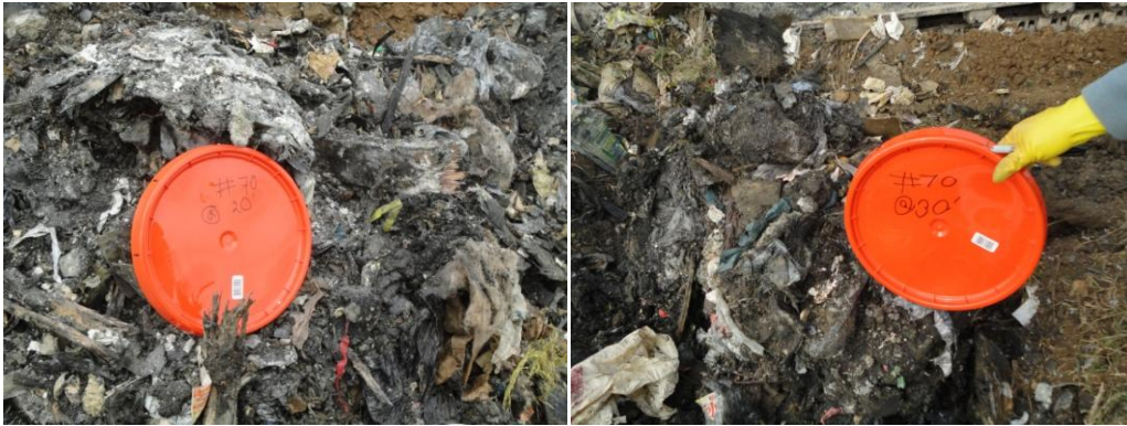
Figure 4.3 Degraded Samples from 20 ft and 30 ft Depth of Boring B-70
