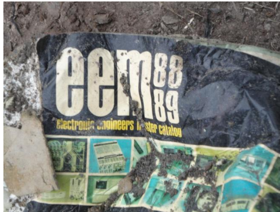
Figure 4.9 Samples with Almost no Degradation from 60 ft Depth of Boring B-72
