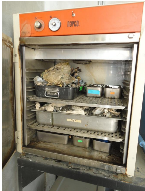
Figure 3.7 Samples Placed in Oven for Determination of Moisture Content
