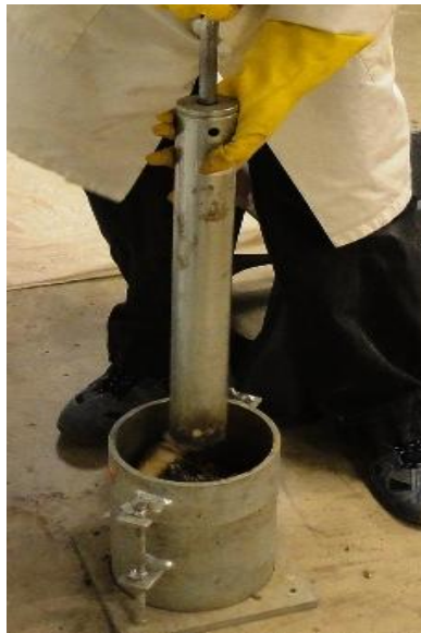
Figure 3.8 Sample Being Compacted
