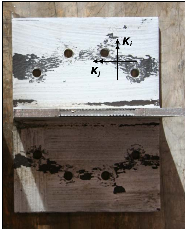
Figure 3-6 Deformed Shape Of The T-Stubs With Circulare Bolt Pattern ( K_i , And K_j Are Curvature In Direction i , And j Respectively)
