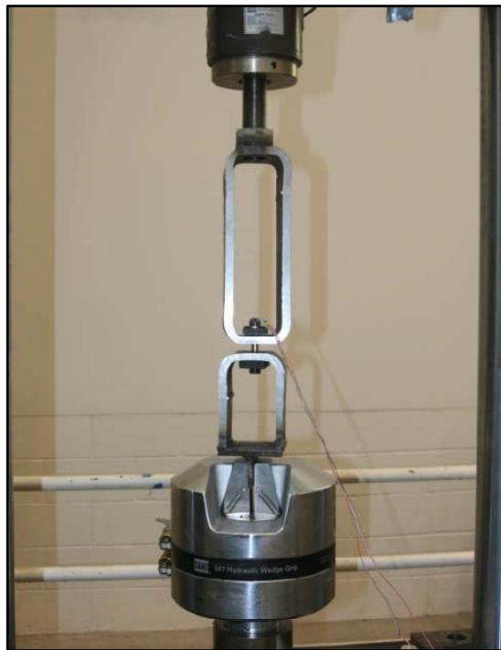
Figure 3-9 Test Setup Used To Verify The Functionality Of The Strain Gauges.
