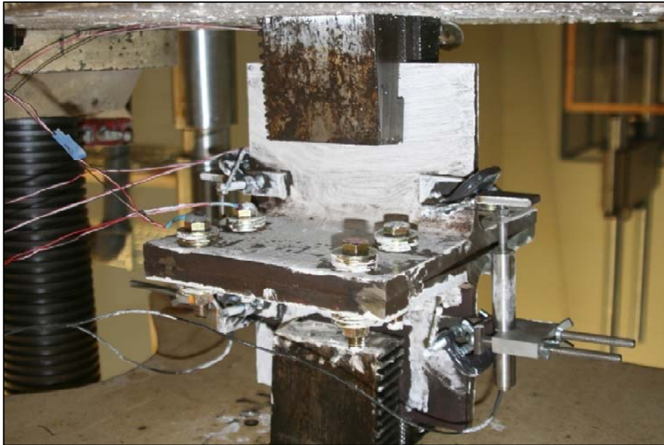
Figure 3-12 T-Stubs Test Setup With Square Bolt Pattern
