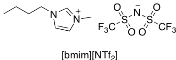
Figure 4.1: The structure and the acronym of 1-butyl-3-methylimidazolium bis(trifluoromethylsulphonyl)imide ionic liquid
