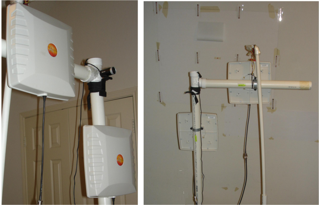
Figure 2.4 Antennas, Web Camera and Tag Mounting on Infrastructure, Front and Back View
