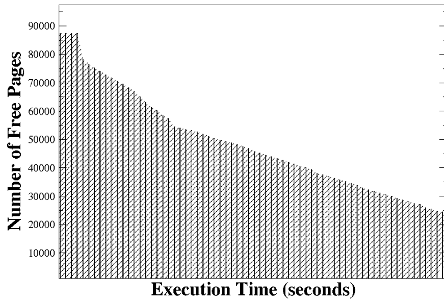
Figure 4.2. Temporal variations of the page pool inside the Virtual Memory (VM) during a typical run of the experiment of Figure 4.1. Notice the availability of free pages inside the VM during the lifetime of the experiment.
