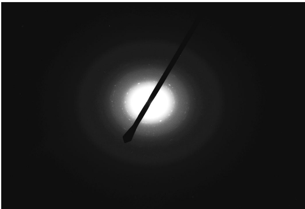
Figure 4.9 SAED pattern of Pt nanoparticles synthesized at 4.1kV using Pt electrodes
