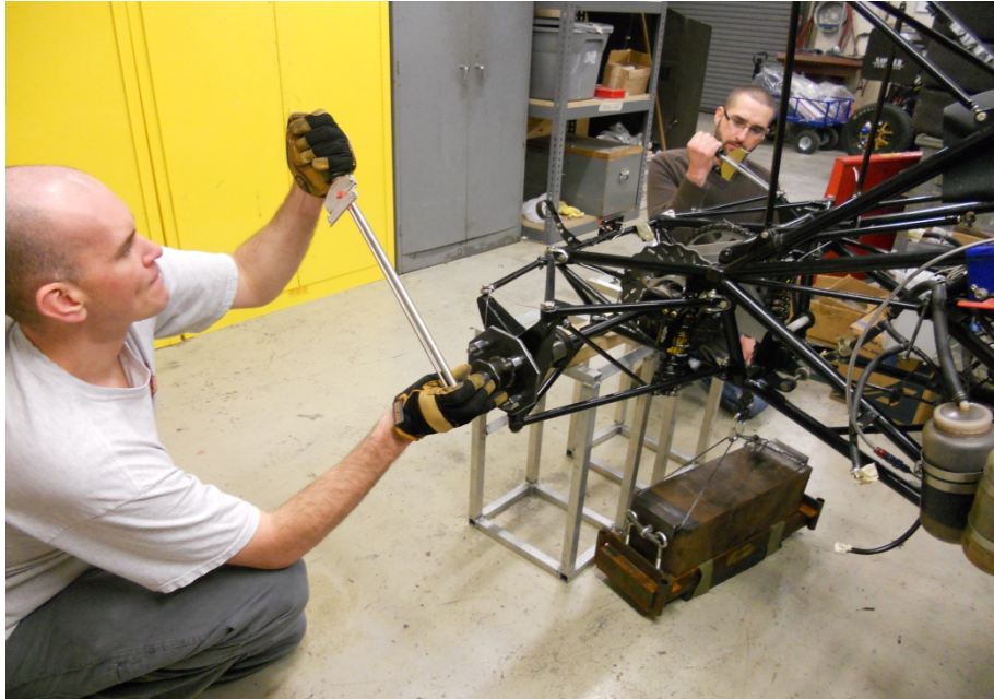
Figure 3.3: The Actual Testing of the Quaife Differential
