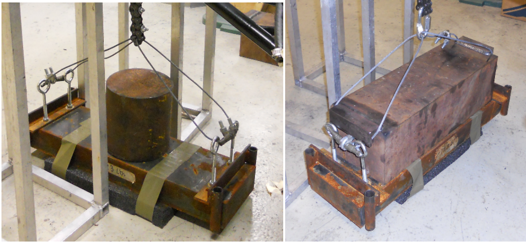
Figure 3.4: The Sled, the Cylinder, and the Steel Block Weights
