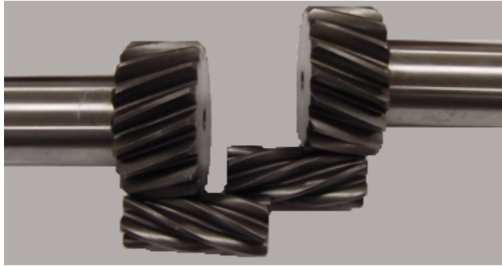
Figure 2.3: Axial Alignment of Planetary Gears to Sun Gears
