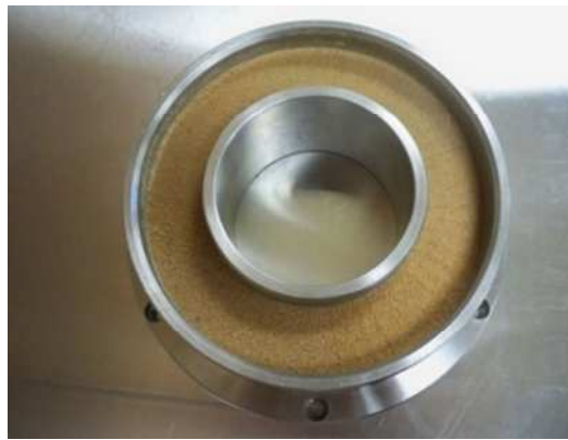
Figure 3-9 Exposed compacted sample of SM.
