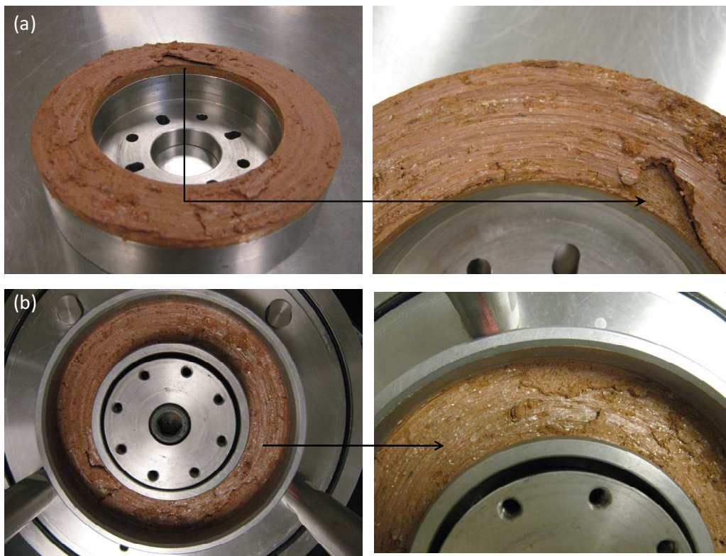
Figure 6-24 Failure plane of SM soil: (a) Top annular platen after shearing and detail of the material adhered to the roughened sintered-bronze porous disk; (b) Bottom annular and detail of the polished, striated failure plane.
