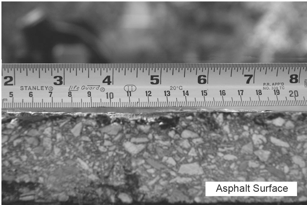
Figure 1.2 Asphalt roadway surface (longitudinal cross-section)
