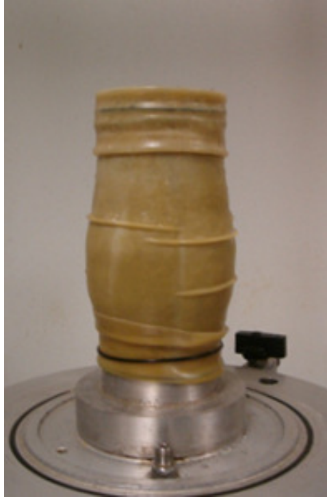
Figure 3.14 Failed Soil Specimen in the Triaxial Test
