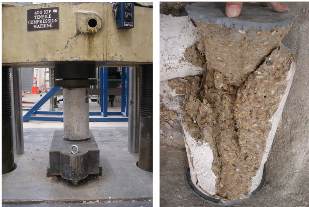
Figure 4.20 Compressive Strength Test Setup and Failed Concrete Specimen
