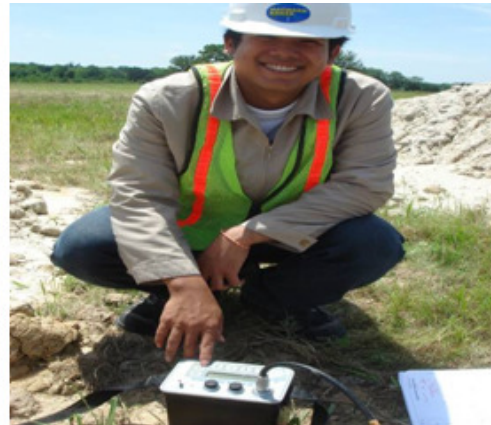
Figure 4.16 Taking Initial Inclinometer Readings
