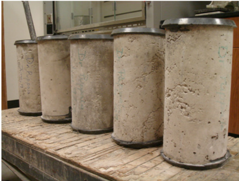
Figure 4.18 Concrete Cylinder Specimens with Capping Compound
