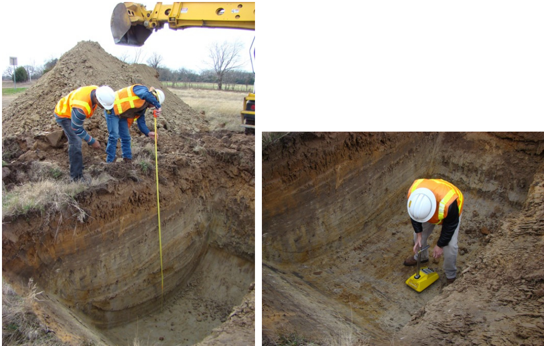
Figure 3.3 Soil Sampling and Density Measurement by Using Nuclear Gauge
