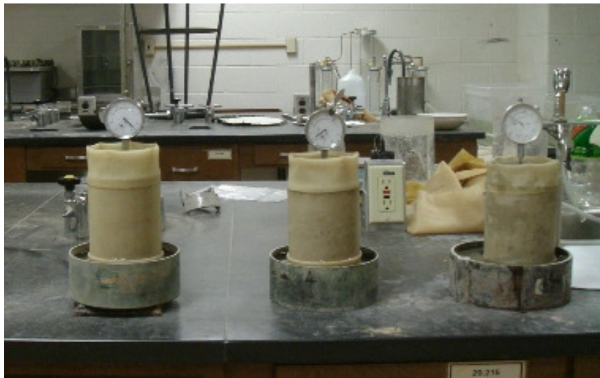
Figure 3.17 Three Dimensional Swell Test of Dry OMC, OMC and Wet OMC Conditions (Left to Right)
