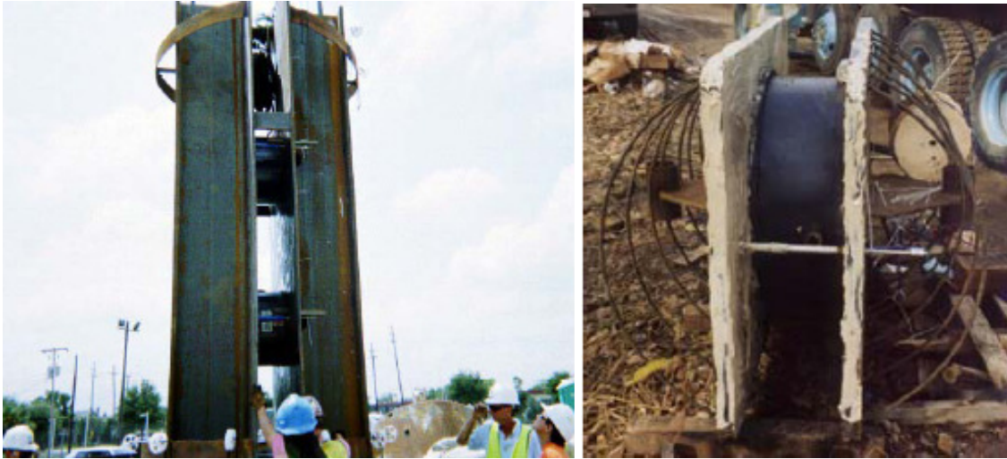
Figure 2.28 Osterberg Load Cell for the Lateral Load Test (Source: http://www.loadtest.co.uk/Loadtest%20Ltd/downloads.htm )
