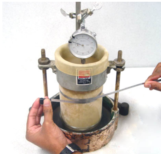
Figure 3.5 Vertical and Radial Measurement for Volumetric Swell Strain
