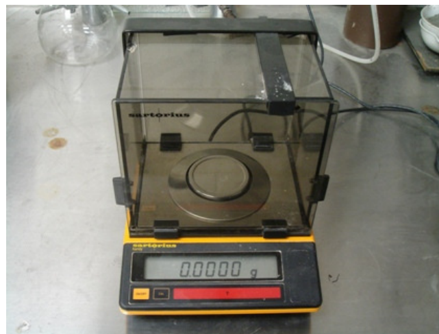
Figure 3.9 Weighing Balance used in Measuring the Weight of the Filter Papers
