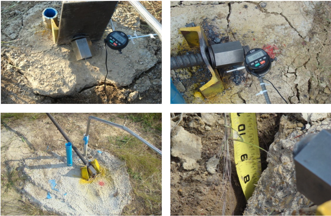
Figure 5.42 Test Shaft Displacements in Summer Condition
