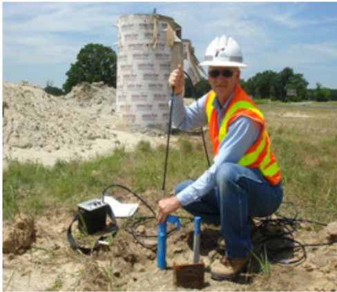
Figure 4.16 Taking Initial Inclinometer Readings
