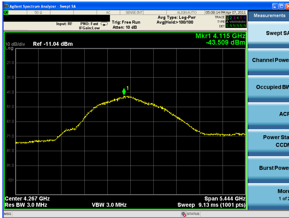
Figure 3.10. Spectrum of UWB pulse in PulsON 220.
