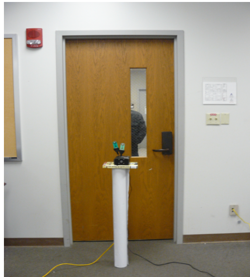
Figure 4.8. UWB Radar in NH 201 and Human target standing outside.
