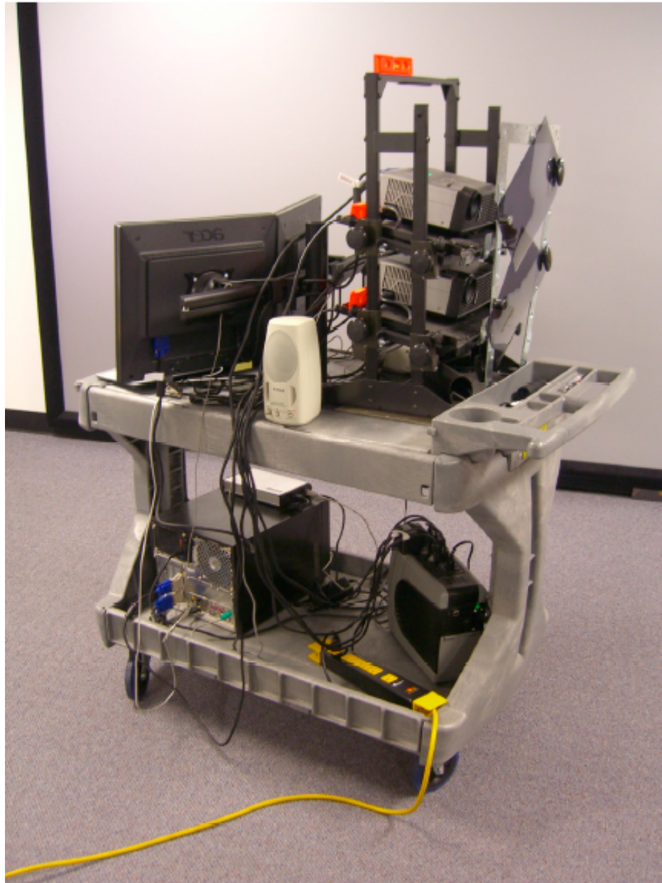
Figure 3.2: GeoWall. The portable GeoWall stereo projection system used in this study (portable silver-matted screen not shown).
