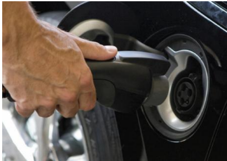
Figure 2.10 PHEV with SAE J1772 standard receptacle about to plug in and charge [22]
