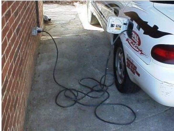
Figure 2.7 Plugging the PHEV on the wall socket with plug and cord set [19]
