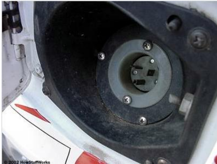
Figure 2.6 Charging plug in NEMA 5-20P configuration shows up by opening the gas filler door [19]
