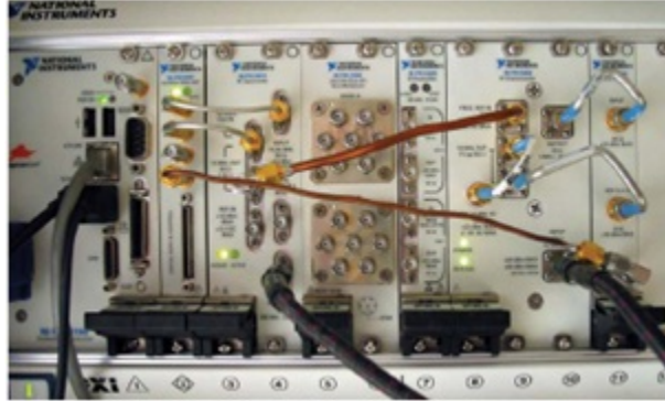
Figure 5.4. Front Panel of the PXI Rack with RFSG and RFSA.
