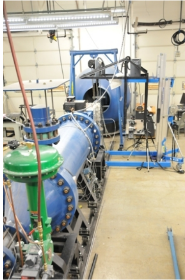
Figure 3.1. Supersonic Windtunnel (SSWT) at the ARC.
