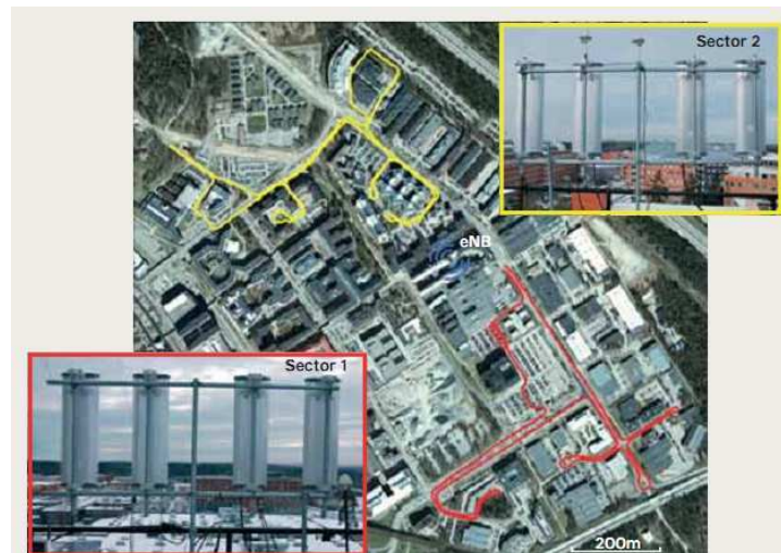
Figure 4.15 The drive routes in Sector 1 (red) and Sector 2 (yellow) each sector as seen from behind the antenna installations [14]
