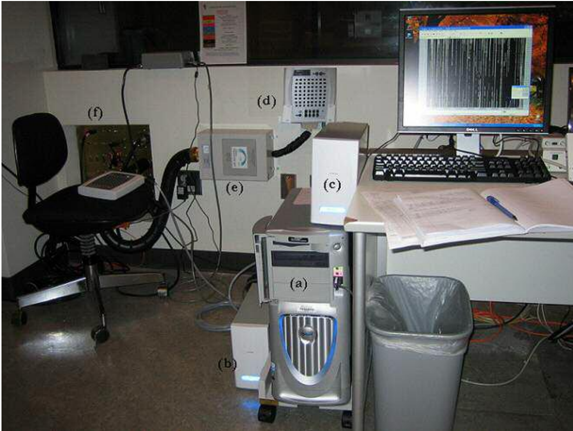
Figure 2.4 Components of the EEG system that are in the control room (a) data acquisition system (b) isolation transformer (c) interface unit (d) amplifier (e) RF filter assembly
