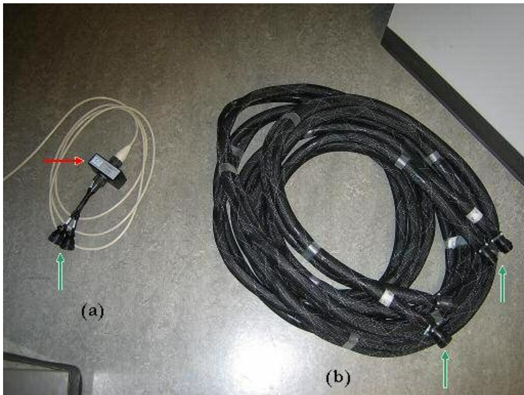
Figure 2.6 Copper - cable (with passive adapter) and the carbon – fiber based cable.
