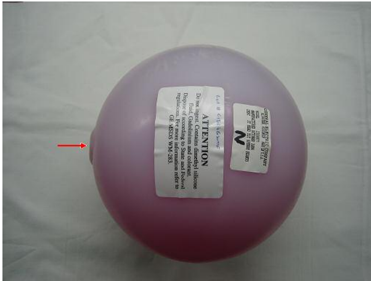
Figure 2.2 Silicone oil phantom used in this thesis project
