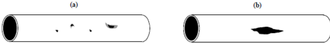
Figure 2.6: (a) Corrosion pitting and (b) Blow-out hole (Misiunas, 2005)
