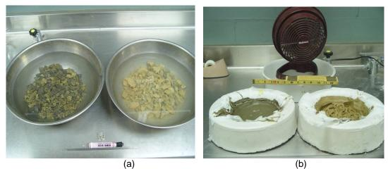
Figure 5.3 Sample preparations by wet analysis for soil classification and determination of Atterberg Limits (a) Soaking stage and (b) Drying stage
