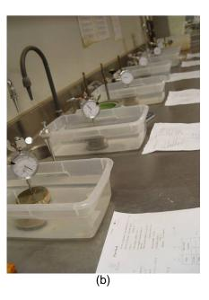
Figure 5.4 Free swell test (a) Schematic Sketch (Das, 2002) and (b) Test Setup
