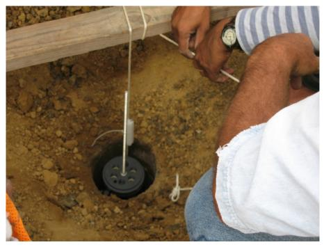
Figure 6.31 The set of assembled rods and reference head was held up by rope
