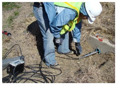
Figure 7.5 Inclinometer data retrieves
