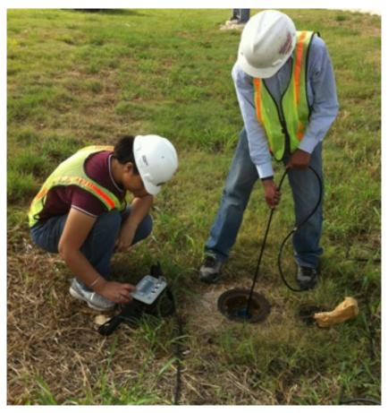
Figure 7.16 The vertical inclinometer reading
