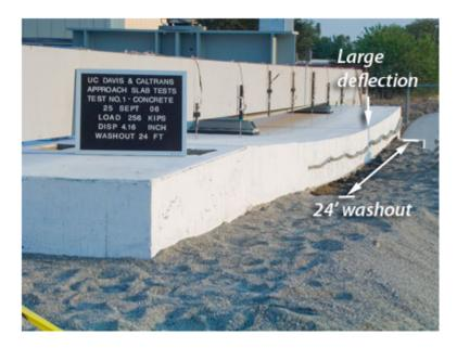
Figure 2.63 Simulated approach slab deflection due to washout by UC Davis research team (<u>http://cee.engr.ucdavis.edu/faculty/chai/Research/ApproachSlab/ApproachSlab.html</u>)
