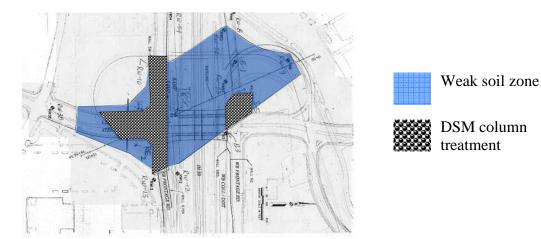
Figure 5.1 Details of weak soil and DSM treatment, IH 30 site, Arlington, TX
