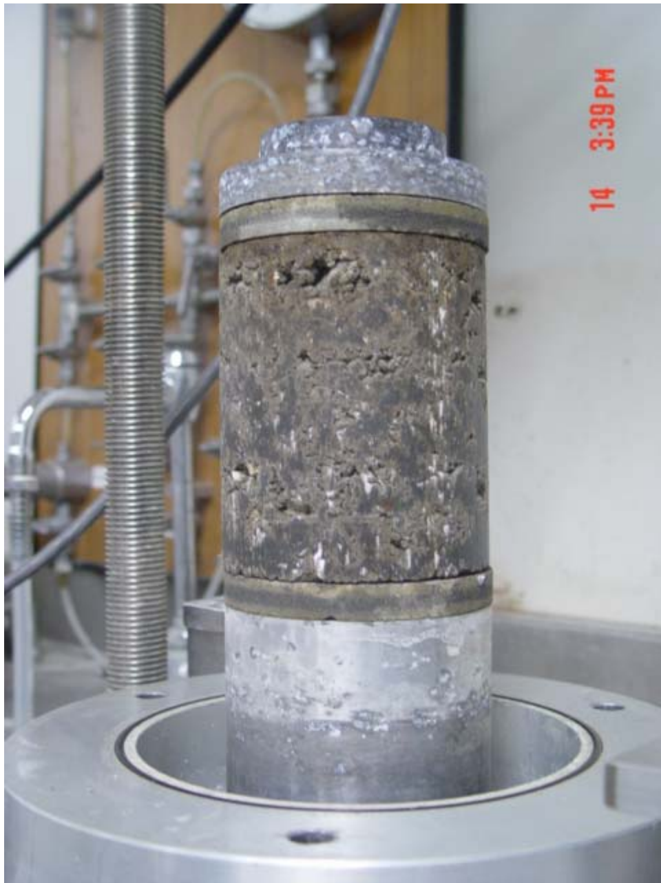
Figure A.2. Specimen Placed on the Triaxial cell for Repeated Load Triaxial Testing
