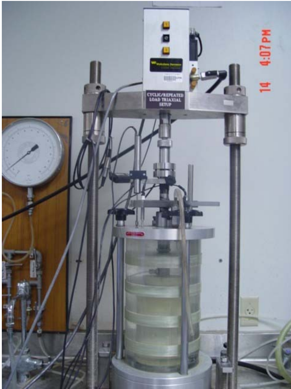
Figure A.4. Specimen Inside the Triaxial Cell
