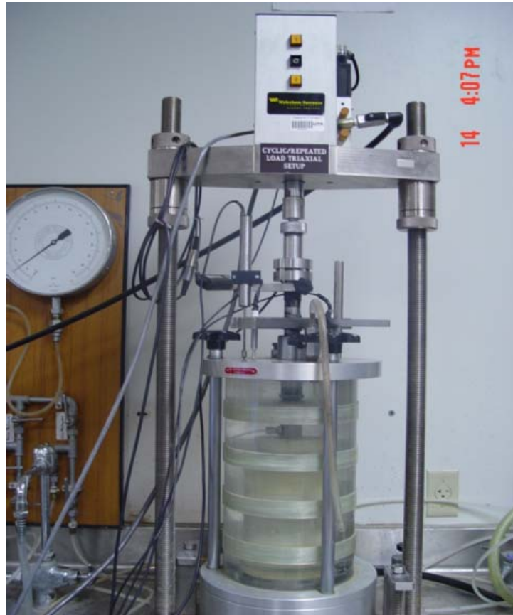
Figure 3.3 The Loading Frame and Triaxial Cell
