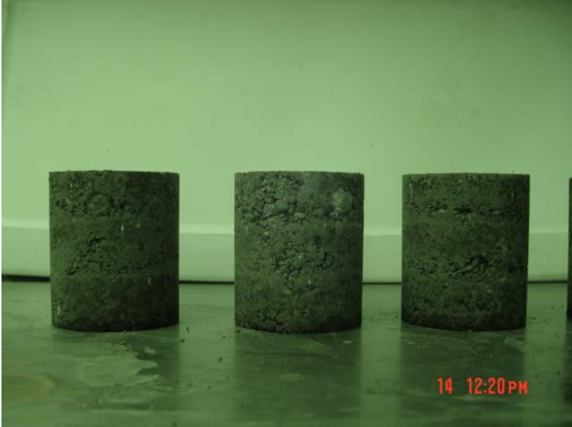
Figure A.1. Compacted RAP Aggregate Material Specimens
