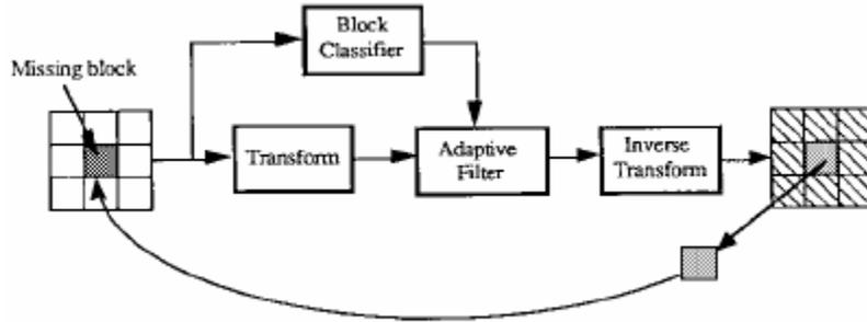
Figure 3.4 Adaptive POCS iterative restoration process [35]
