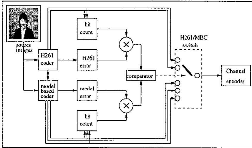
Figure 4.2 System diagram of high level switching [58]
