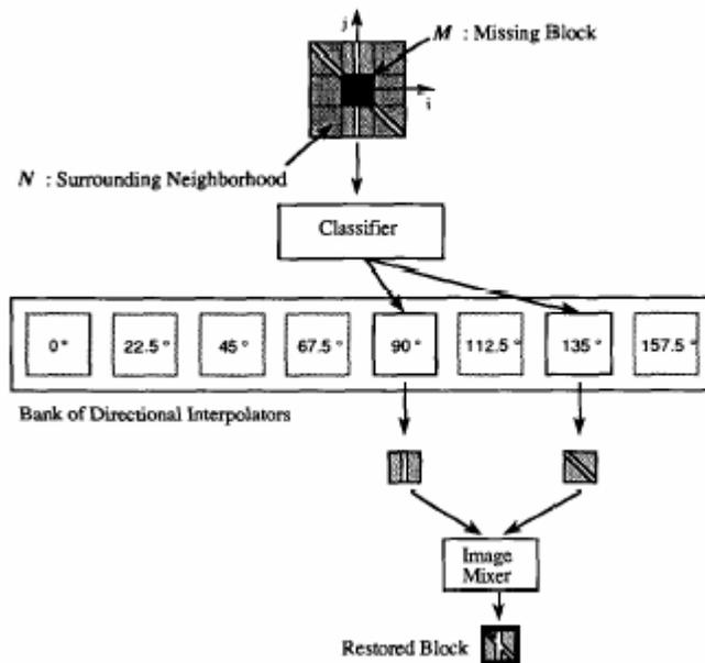
Figure 3.2 Illustration of multiple directional interpolation algorithm [33]
