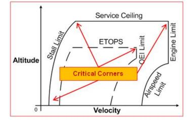
Figure 4.2 A typical flight envelope and the some critical corners
