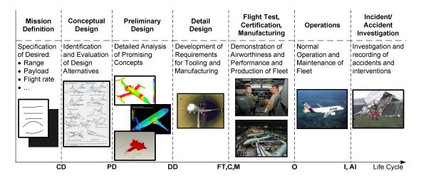
Figure 1.1 Aircraft Lifecycle as described in the AVD Lab
