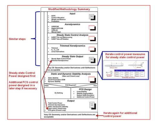
Figure 5.1 AeroMech methodology showing iteration steps for control power
