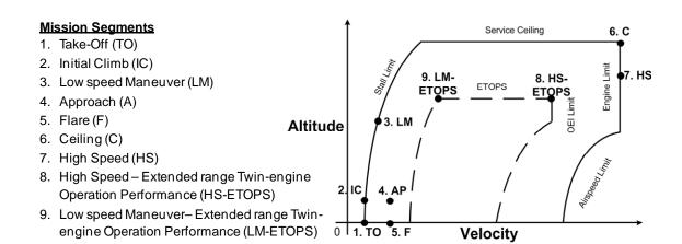
Figure 5.3 Critical corners of the flight envelope for control power assessment of a TVC transport
