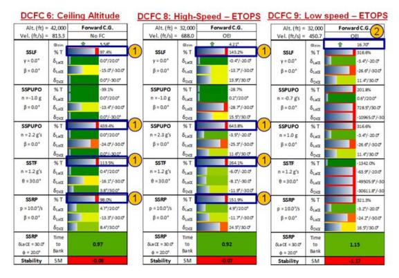
Figure 5.9 Control power assessment chart for engine limit conditions
