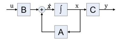
Figure 2.1 Block diagram of aircraft linear time invariant model
