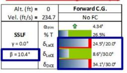
Figure 5.8 Control power assessment chart for segments with maximum crosswinds
