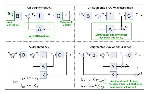
Figure 2.4 block diagrams showing increase in control power requirement
