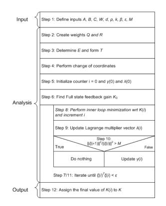
Figure 3.1 Summary of algorithm for constrained output feedback of similar system
