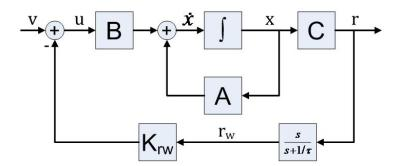
Figure 2.6 Block diagram of a yaw damper with a washout filter.
