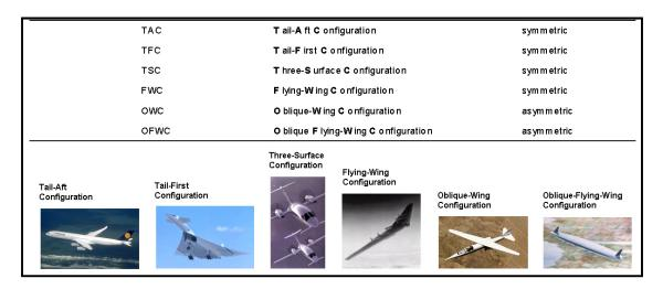
Figure 1.5 Aircraft configurations (Chudoba 2001)
