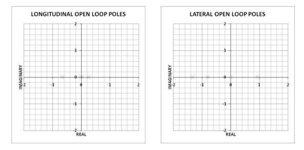
Figure 5.10 Longitudinal and lateral-directional open loop poles plots for the TVC transport
