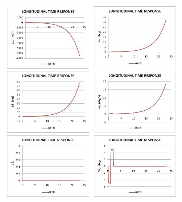
Figure 5.11 Open loop time response of the TVC transport to a 5 deg elevator doublet
