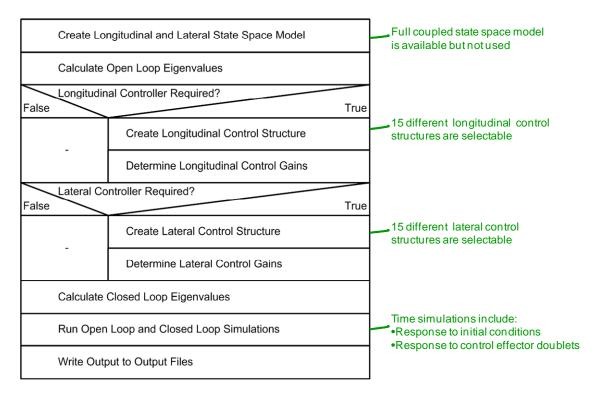
Figure 4.6 Details of the FCS module
