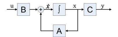
Figure 2.2 Block diagram of aircraft LTI model with feedback control
