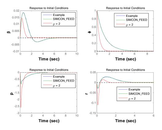
Figure 3.5 Response of system design with proposed algorithm to initial bank angle
