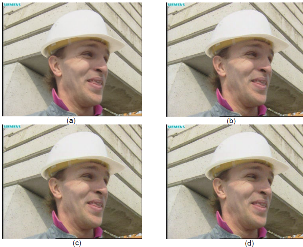
Figure 6.23 Foreman sequence (a) Original (b) H.264 decoded (c) Reference cascade decoded at QP 10 (d) Proposed transcoder decoded at QP 10
