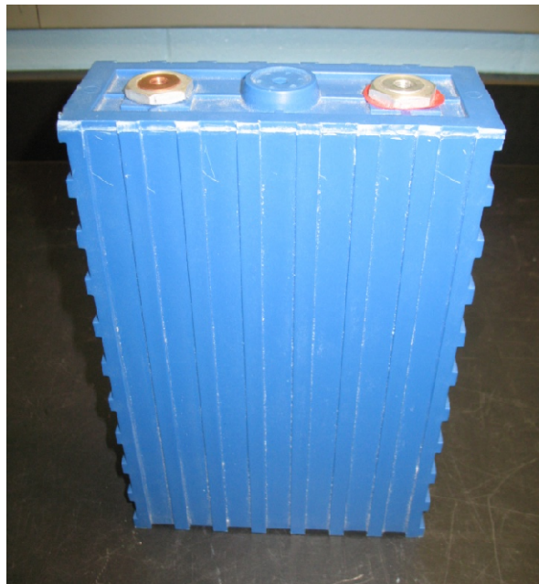
Figure 4.12 The SE180AHA Li-Ion battery specifications. (a) battery specifications and (b) the experimental battery.
