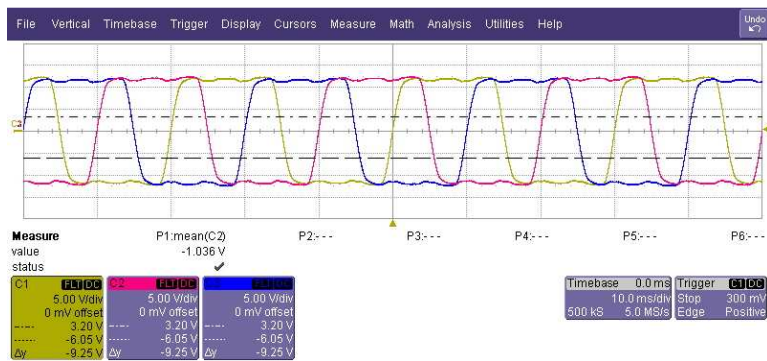
Figure 4.2 Back-EMF of PMSM at 1000 rpm from PMSM
