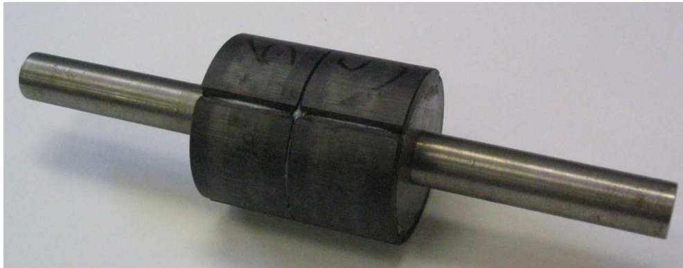
Figure 2.7 Structure of 4-poles rotor with permanent magnet at the surface
