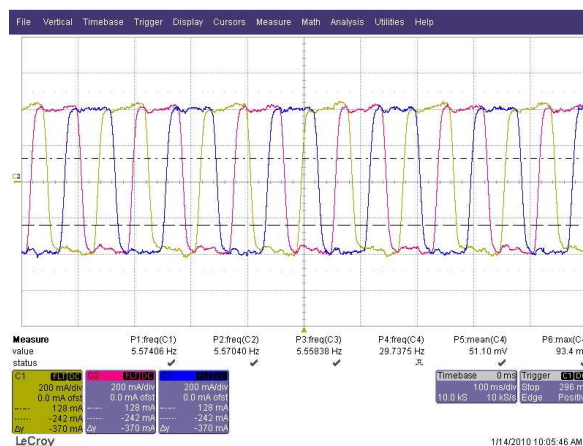
Figure 4.6 Three-phase current supplied to the load of PMSM at 167 rpm
