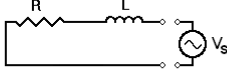
Figure 2.8: Equivalent circuit model for phase winding of the PMSM.
