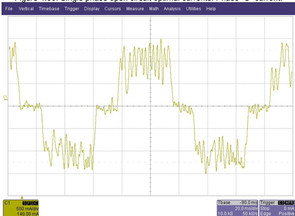
Figure 4.31: Double phase open circuit optimal currents: Phase “A” current.
