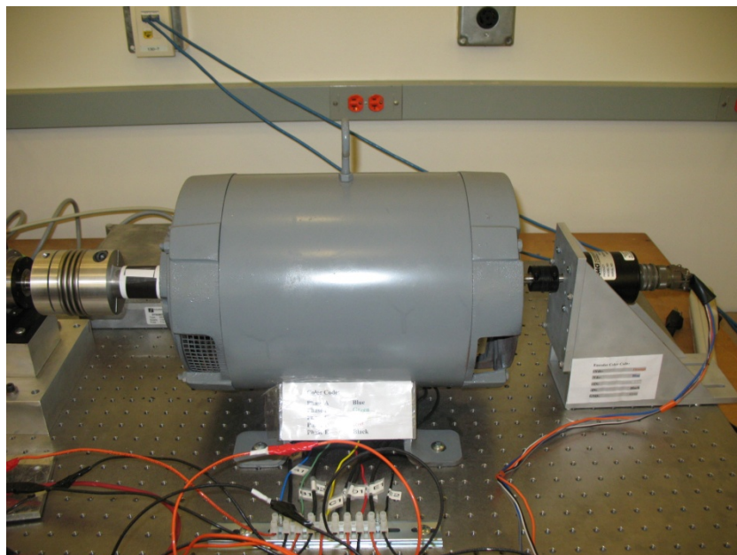
5-phase PMSM coupled to the absolute position encoder
