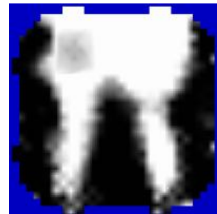
Figure 6.7. Simulated Millimeter Wave Sensor Image Showing the Lower Region of a Person with an Metal Plate in Right Thigh.
