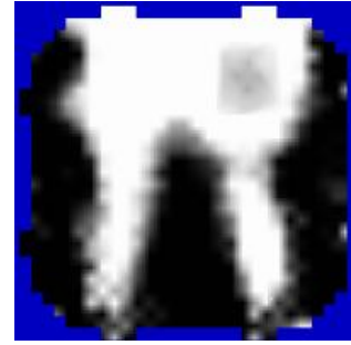
Figure 6.9. Simulated Millimeter Wave Sensor Image Showing the Lower Region of a Person with an Metal Plate in Left Thigh.
