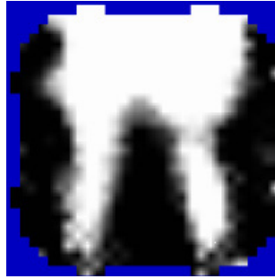
Figure 4.5. Simulated Millimeter Wave Sensor Image Showing the Lower Region of a Person With a Gun in The Right Abdomen.
