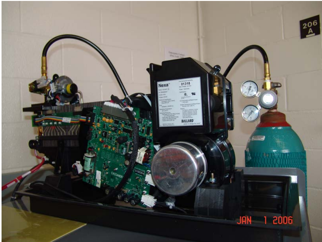
Figure-1.1 Experimental fuel-cell setup used for implementation and analysis
