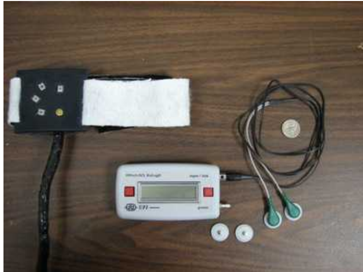
Figure 5.1 Biolog 3991x/1 system and the electrodes being used along with the LCC – NIRS probe
