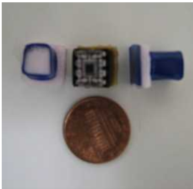
Figure 2.6 Picture of the top and side views of the detector moulds with the model of an actual detector
