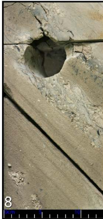
3891.7m - Mud rip up layers in cross-bedded sand.
