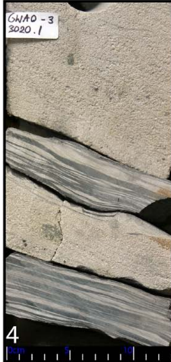
4 ~3020.2m - Ripple scale mud drapes in active channel.
