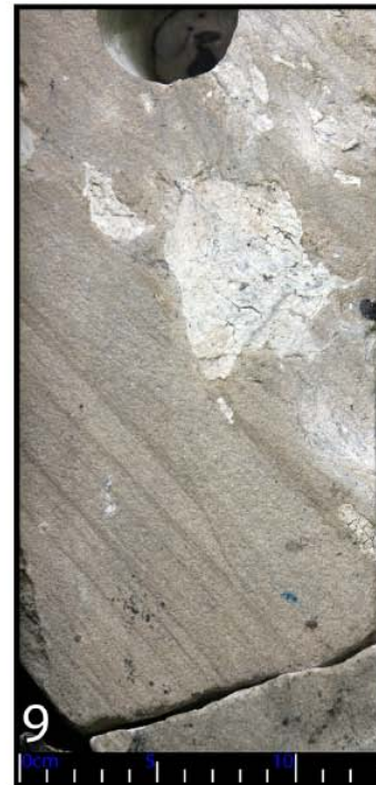
3893.9m - Isolated mud ball in cross-bedded sand.
