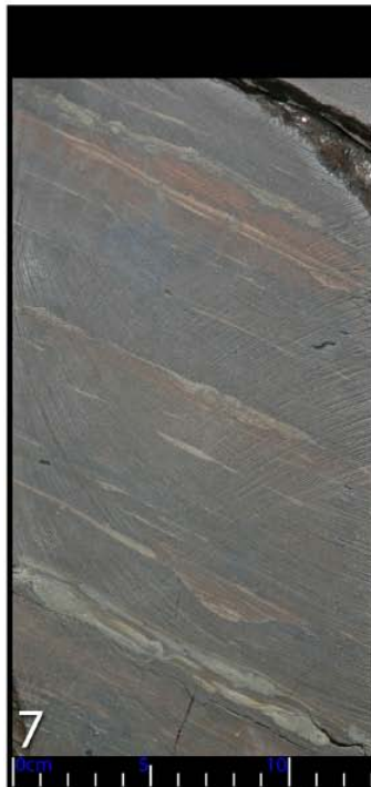
7 ~3030.8m - Hyperpycnal scour with ripple scale bed forms into open lake.
