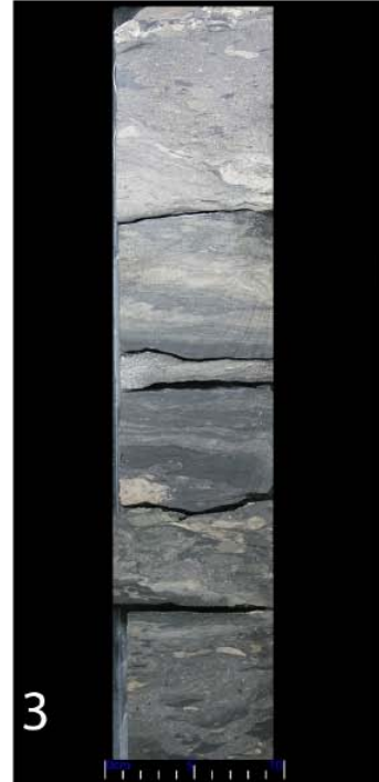
2884.9m - Rippled sand with mud drapes and mud rip-ups.
