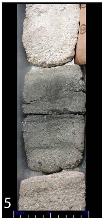
~2887.8m - Muddy sand cap or drilling Mud?
