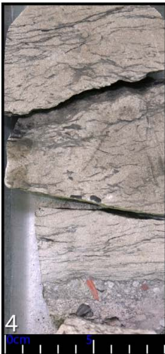
2885.3m - Mud rip-up conglomerate and silty ripples.
