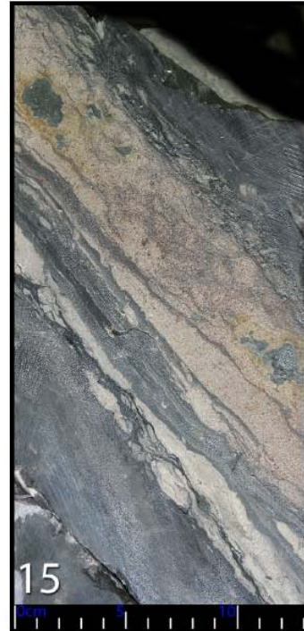
15 3927m - Small splay delta within boggy to lake transition. Bioturbation at base of splay and thin coaly lamina at top.
