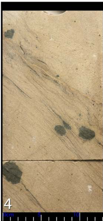
3875.2m - Mud balls in wavy laminated sand.
