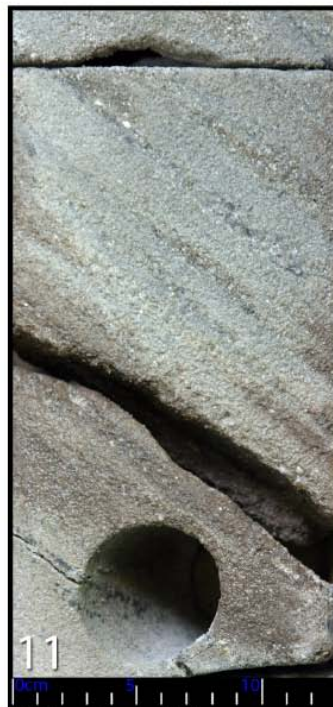
3905.5m - Cross-bedded coarse sand. Active channel fill.
