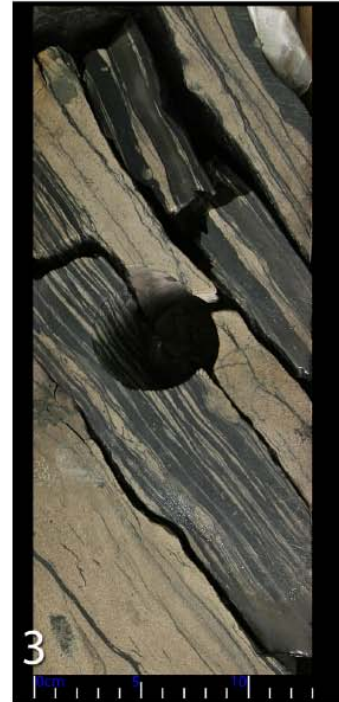
3873.8m - Couplet set with rippled sand and mud drapes. Another couplet set at 3874.3m.
