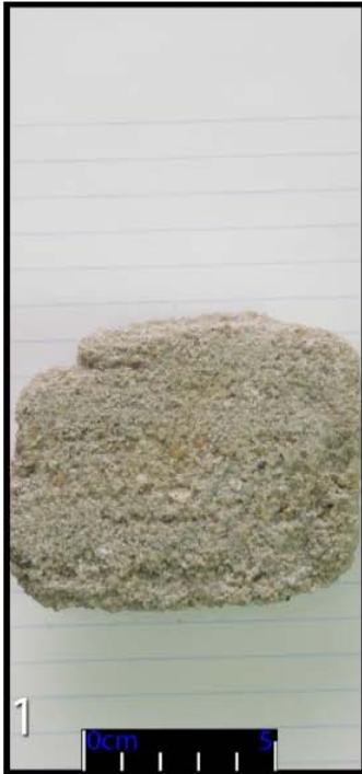
2846.6m - Granular cross-bed between two slightly less granular parallel laminated sets.
