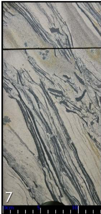
3889.7m - Scour surface in rippled sand.
