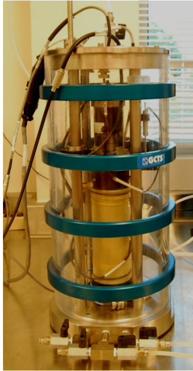
Figure 3-8 Proximito-based RC Main cell
