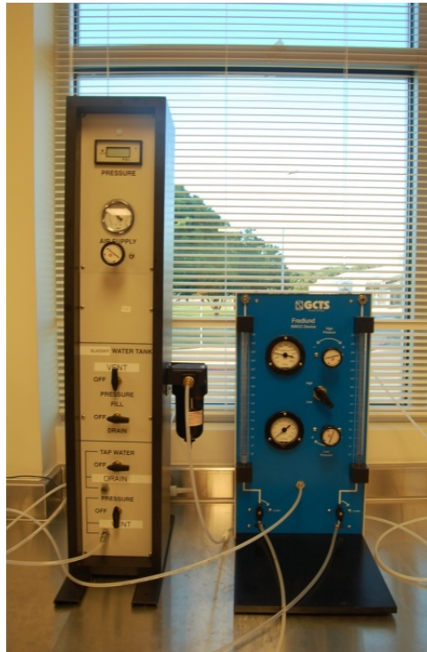
Figure 4-2 Pressure control panels
