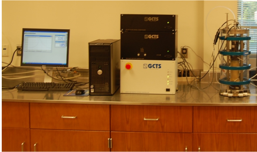
Figure 3-7 General layout of the proximator-based RC device
